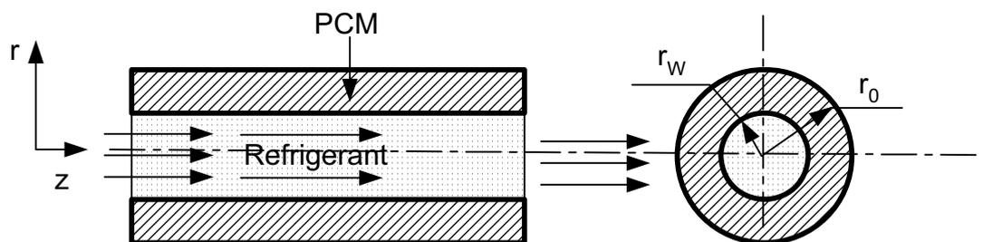
Figure 1: Thermal energy unit and its cross sectional view
