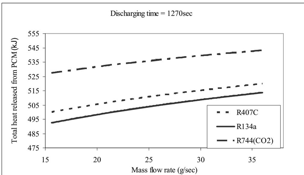
**Figure 11: Effect of mass flow rate on total amount of heat released**
