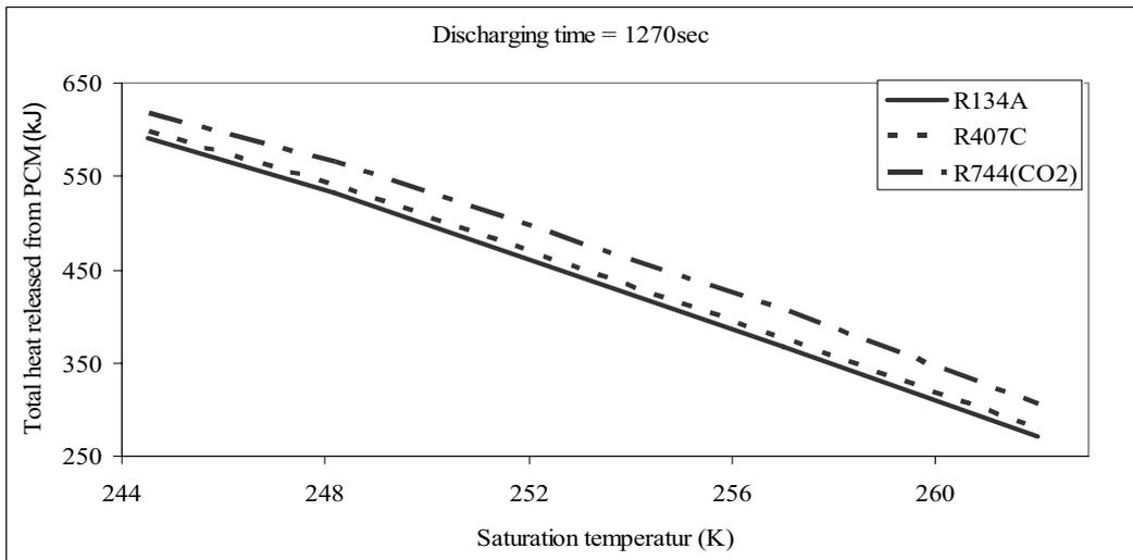
**Figure 10: Effect of the saturation temperature of fluid on the total heat transfer released from PCM**
