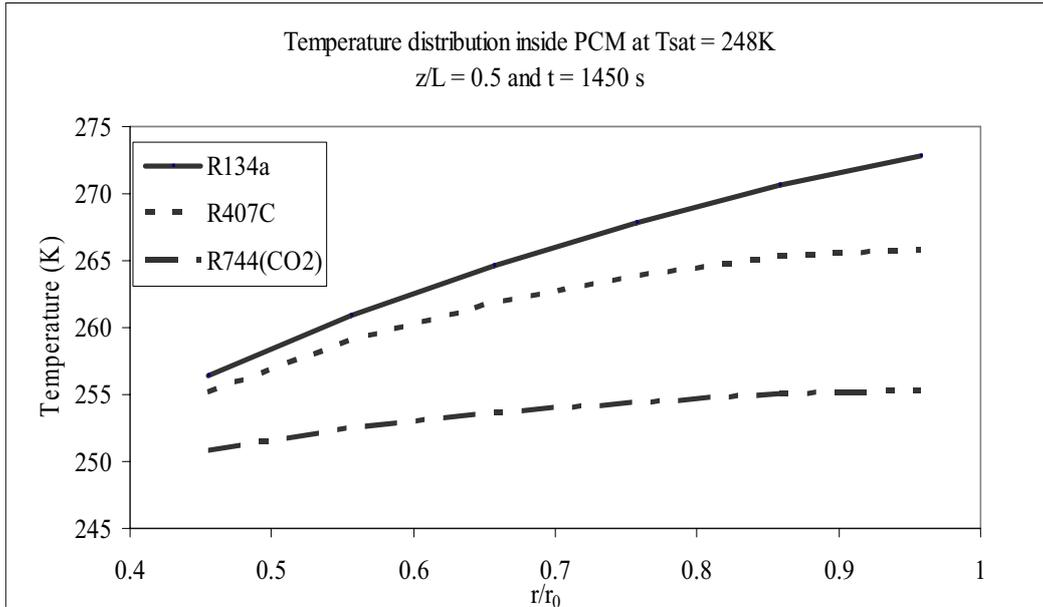
**Figure 6: Effect of saturation temperature of Refrigerants flow on the temperature distribution inside the phase change material (Tsat = 248K)**
