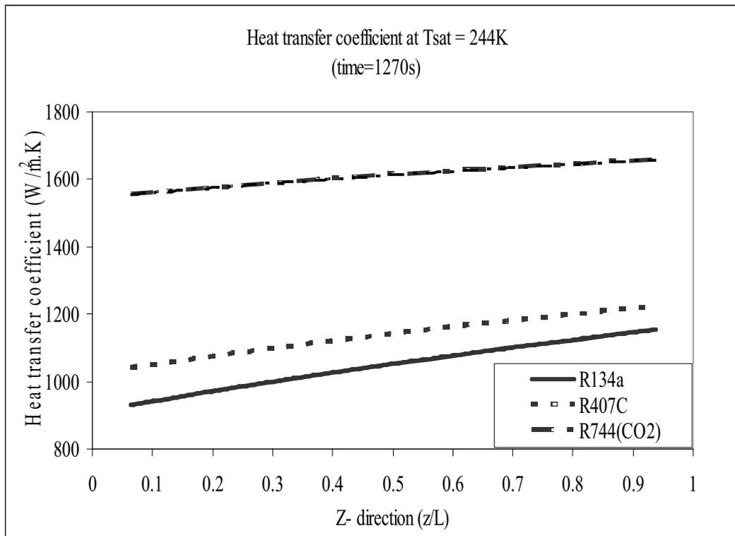
**Figure 3: Variation of heat transfer coefficient in the axial direction**
