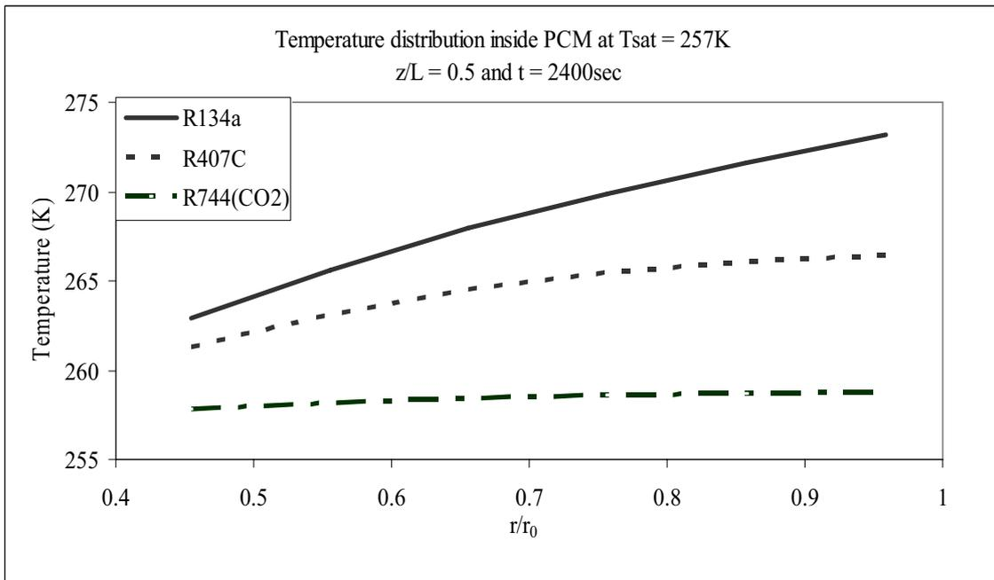
**Figure 7: Effect of saturation temperature of Refrigerants flow on the temperature distribution inside the phase change material (Tsat = 257K)**
