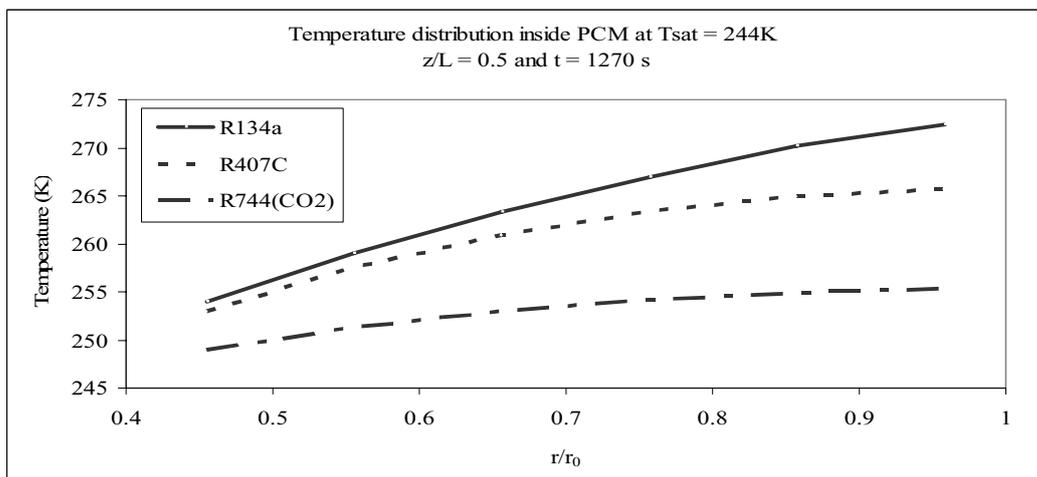
**Figure 5: Effect of saturation temperature of Refrigerants flow on the temperature distribution inside the phase change material (Tsat=244K)**
