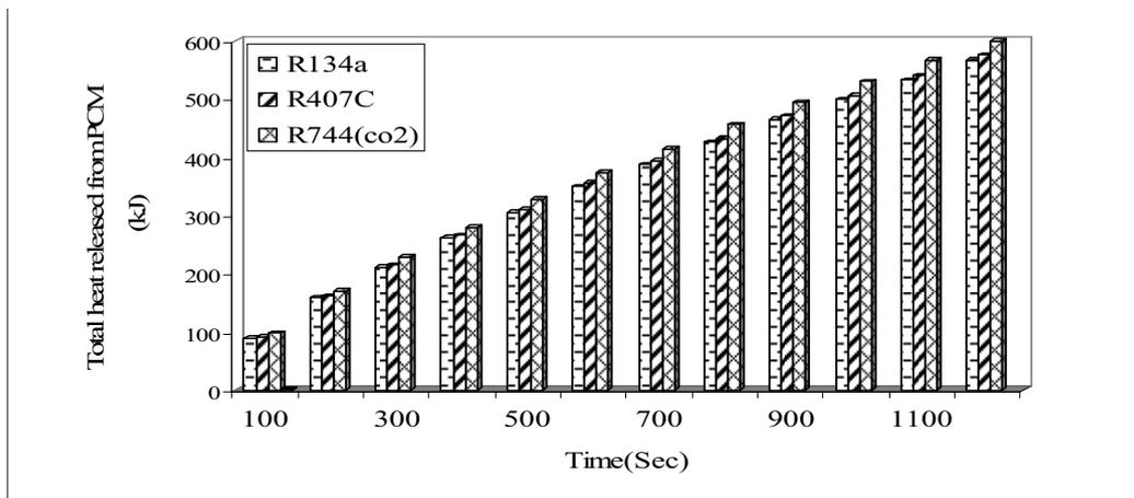
**Figure 9: Time effect on the total heat released from PCM**
