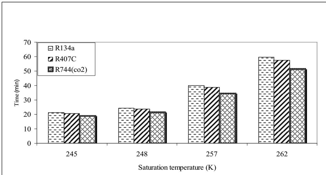
**Figure 4: Effect saturation temperature on the time solidification of PCM**
