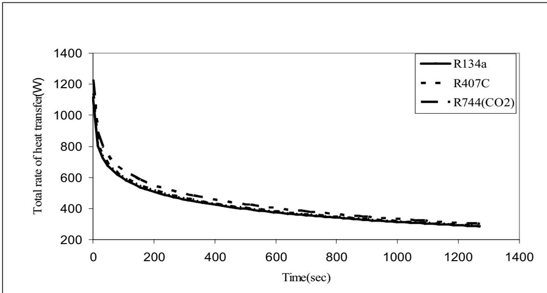
**Figure 8: Time effect on the total heat rate absorbed by the refrigerant**
