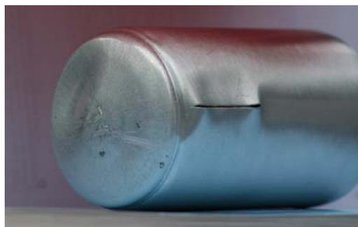
**Figure 17: Deformation and burst pressure of can base**
