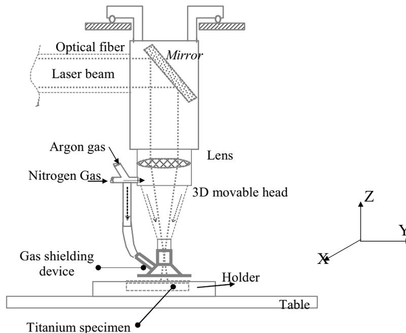
**Figure1: A schematic diagram of the laser nitriding experimental setup.**
