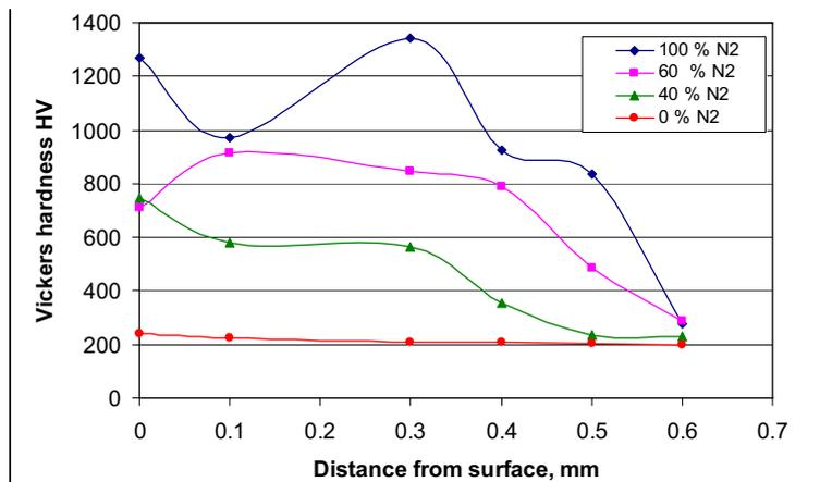
**Figure 9: Microhardness profiles across the nitrified layer produced on CP Ti at different nitrogen concentrations.**
