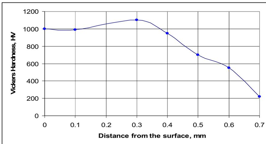
**Figure 7: Microhardness profile across the nitrided layer produced on CP titanium by a laser power of 3 kW, 100 %  $\text{N}_2$  and a scanning rate  $V = 900$  mm/min.**
