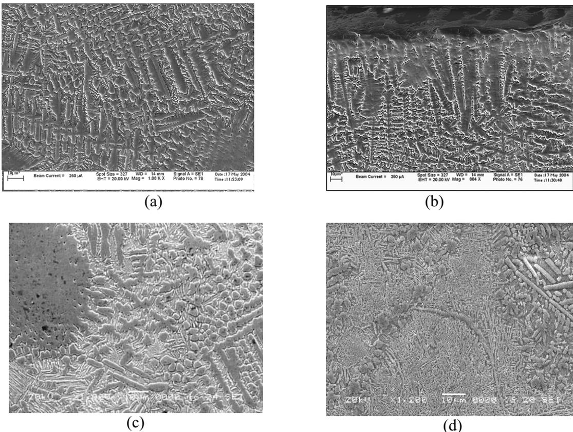
**Figure 3: SEM micrographs of various zones of the nitride track cross-section: (a) the upper zone; (b) the central zone; (c) the left side; (d) the N-free zone.**
