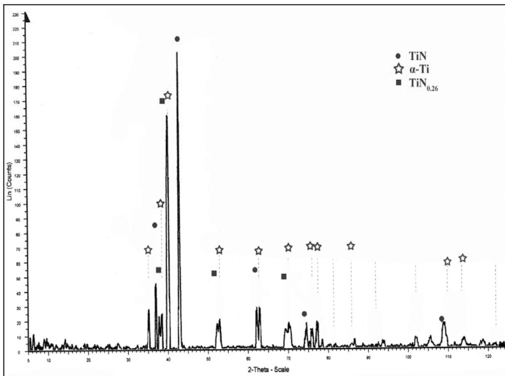
**Figure 5: X-ray patterns taken from the nitride layer at a depth  $100 \mu\text{m}$  from the surface (2.5kW, 17 l/min. 900 mm/s, and 100% nitrogen).**
