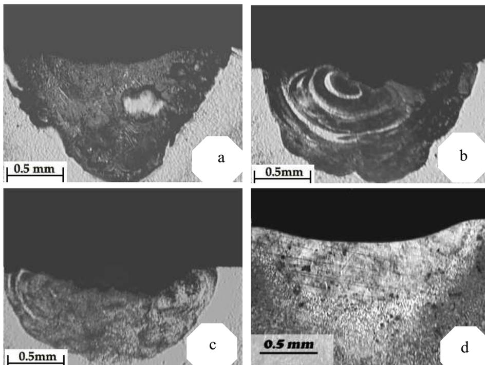
**Figure 8: Optical micrographs of nitride layers at different nitrogen content in the nitrogen/argon gas mixture (a) 100% N<sub>2</sub>, (b) 60% N<sub>2</sub> (c) 40% N<sub>2</sub>, and (d) 100% Ar.**
