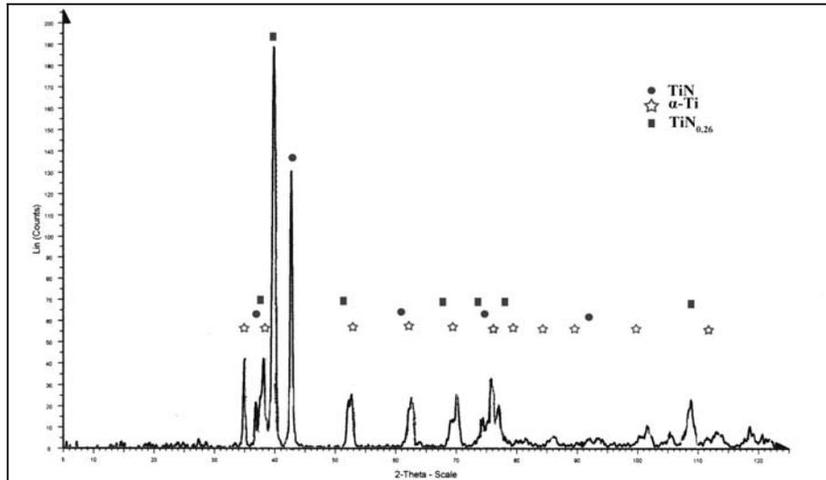
**Figure 6: X-ray patterns taken from the nitride layer at a depth 300  $\mu\text{m}$  from the surface.**
