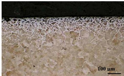
**Figure 8: Optical micrograph of longitudinal section of the rail gauge face (GL) for new rail P5. Moving down the picture there is sample mounting material, top rail surface containing a small grain size with large amount of ferrite and the bulk material microstructure.**
