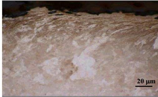
**Figure 7a: Optical micrograph of longitudinal section of the rail gauge face (specimen GL) for rail P4. Moving down the picture there is sample-mounting material; large deformed steel microstructure is visible**
