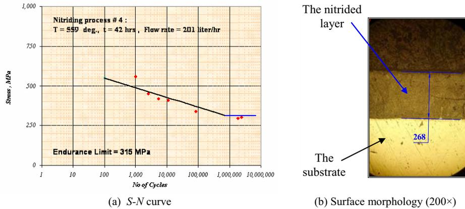
**Figure 6: S-N curve for fatigue test and layer morphology of nitrided specimen (Design point No 4 (T = 559 °C, t = 42 hrs , Flow rate = 201 liter/hr))**
