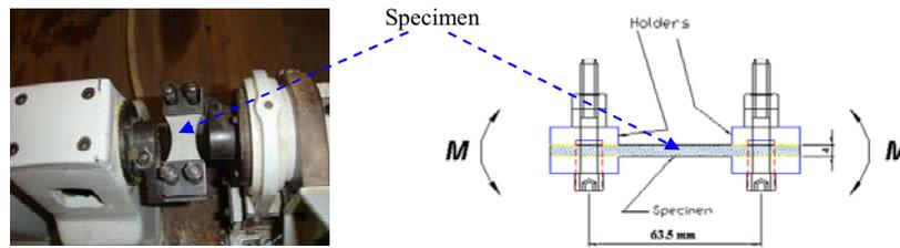
Figure 5: The pure bending loading condition of the smooth samples
