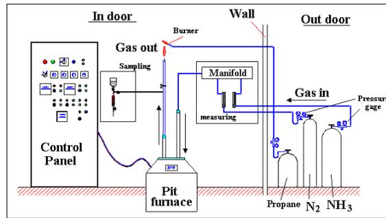
**Figure 2: Gas nitriding Pit Furnace model 572 (SIB company)**
