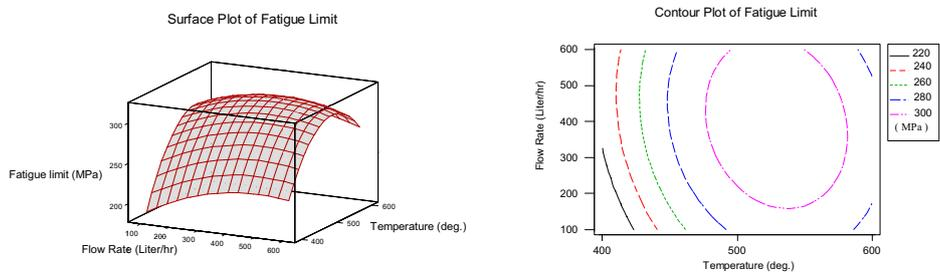
(c) 3D plot and contour for fatigue strength with nitriding temperature and flow rate
