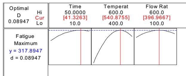
Figure 8: Optimization chart of gas nitriding process for maximum fatigue strength
