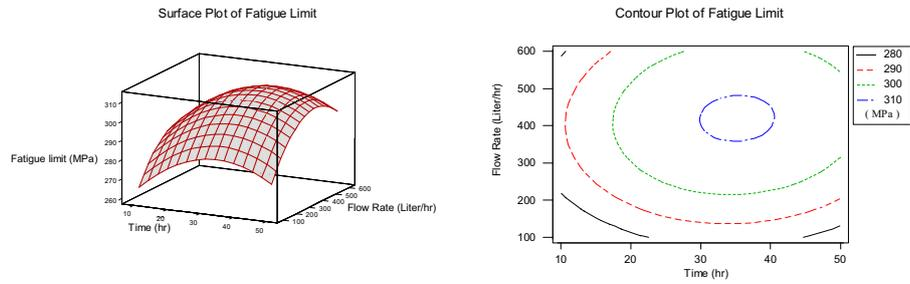
(b) 3D surface plot and contour for fatigue strength with nitriding time and ammonia flow rate
