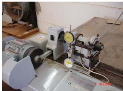
**Figure 4: Avery-Denison fatigue testing machine**
