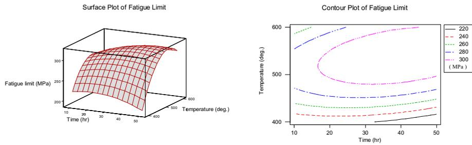
(a) 3D surface plot and contour for fatigue strength with nitriding time and temperature
