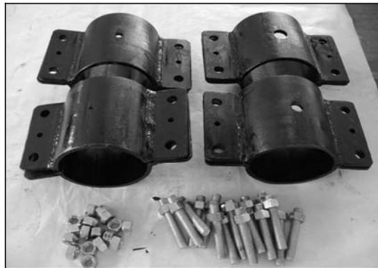
Figure 3: Bolted steel clamps
