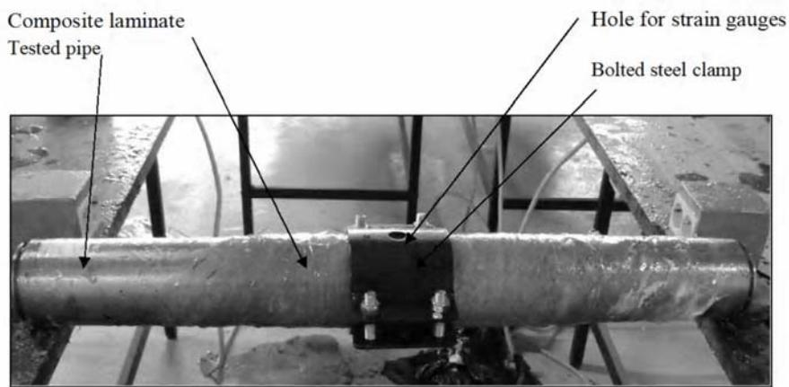
**Figure 5: A repaired pipe with bolted steel clamp**
