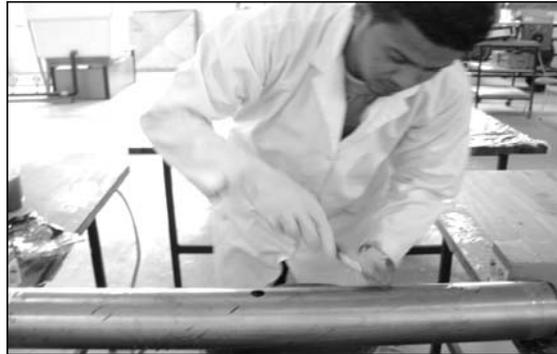
**Figure 4: The beginning of the over wrapping the pipe with layers of fiber glass**
