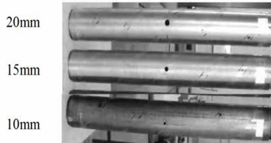
Figure 2: Specimens of pipes with defected holes of 10, 15 and 20mm
