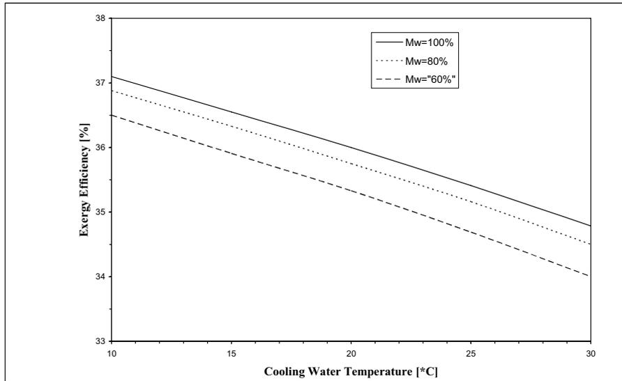
**Figure 7: Variation of exergy efficiency with inlet cooling water temperature at different cooling flow rates.**
