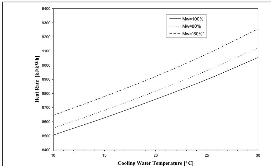
**Figure 6: Variation of heat rate with inlet cooling water temperature at different cooling flow rates.**
