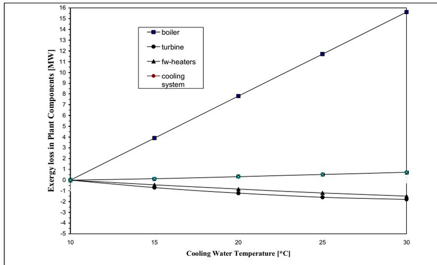
**Figure 9: Variation of exergy destruction in plant components with inlet cooling water temperature at different cooling flow rates.**
