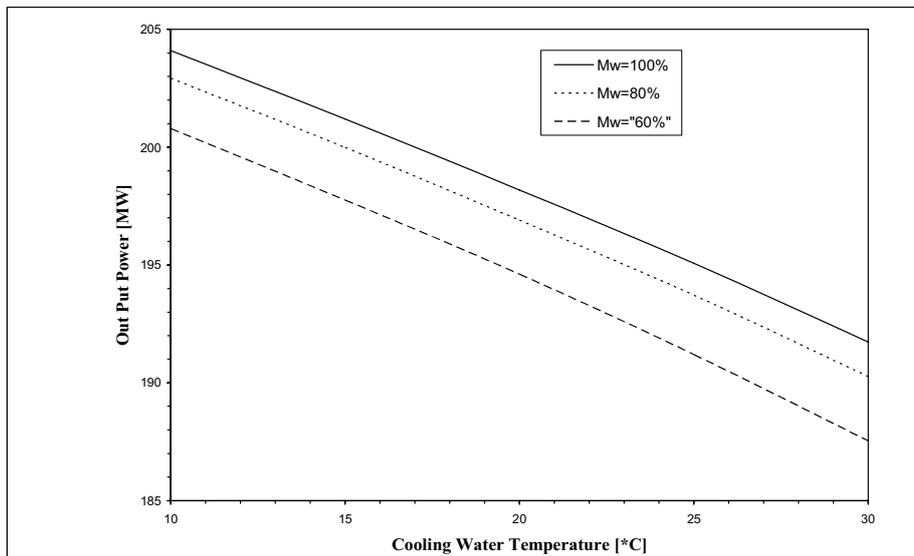
**Figure 5: Variation of out-put power with inlet cooling water temperature at different cooling flow rates.**
