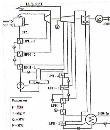
Figure 1: Schematic diagram of 200 MWe steam cycle power plant.
