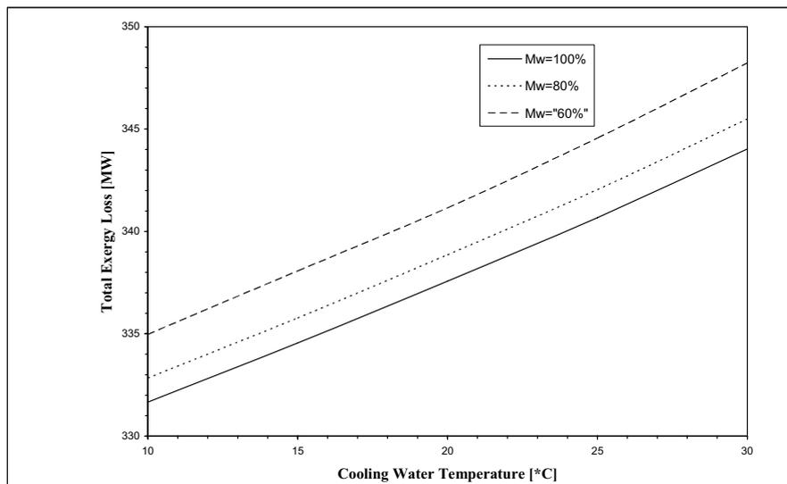
**Figure 8: Variation of total exergy destruction with inlet cooling water temperature at different cooling flow rates.**
