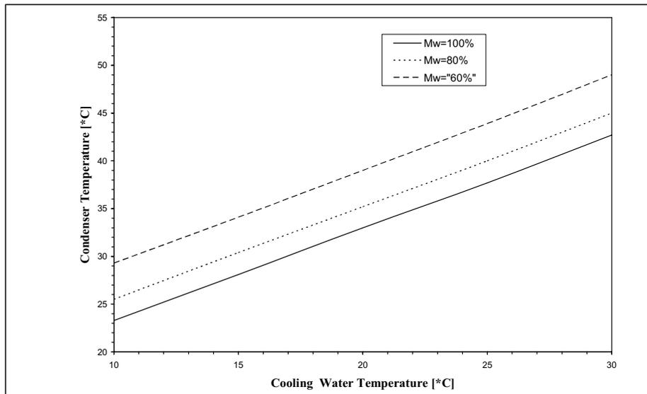
**Figure 4: Variation of condenser temperature with inlet cooling water temperature at different cooling flow rates.**
