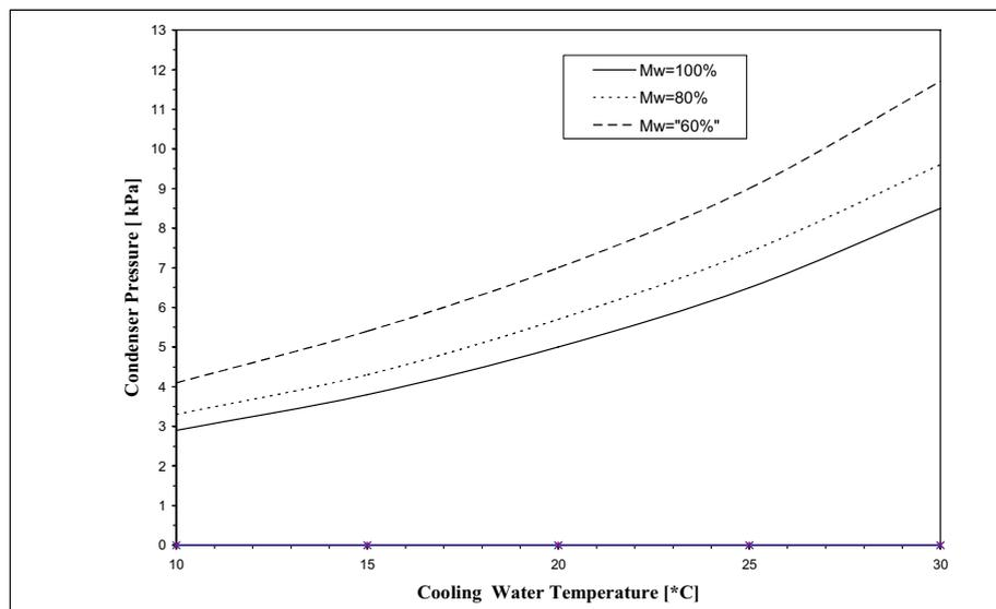
**Figure 3: Variation of condenser pressure with inlet cooling water temperature at different cooling flow rates.**
