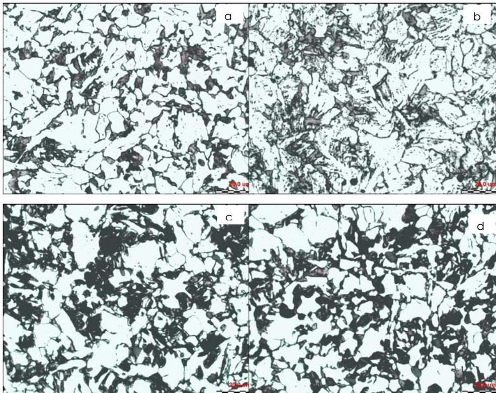
Figure 3: Typical light microscopy images of dual-phase steels showing dispersion of martensite (black block), and ferrite (white). Micrographs (a), (b), (c) and (d) correspond to the microstructures obtained with IQ at 730, 750, 775 and 800°C, respectively.
