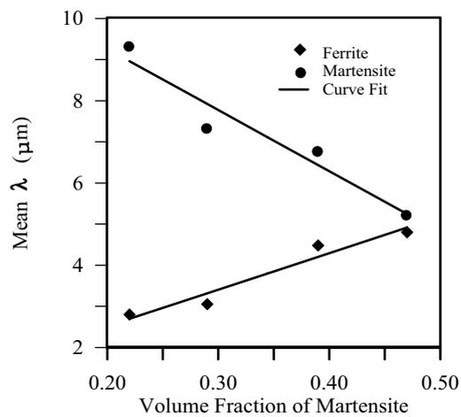
Figure 4: Mean intercept of ferrite and martensite grains plotted against the volume fraction of martensite
