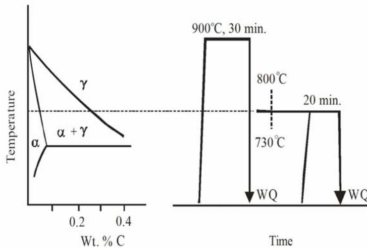
**Figure 2: Schematic representation of heat treatment schedules IQ treatment**
