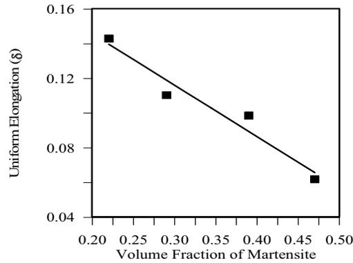
**Figure 7: Effect of the martensite volume fraction on the uniform deformation extent**
