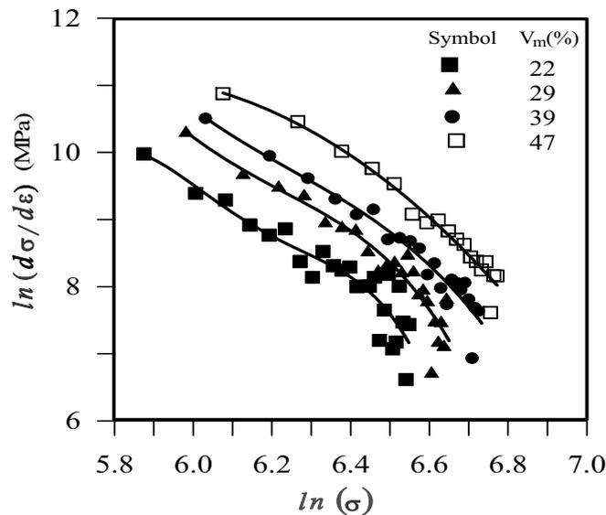
**Figure 8: Representative experimental  $\ln(d\sigma/d\varepsilon)$  versus  $\ln(\sigma)$  curves for different volume fractions of martensite**
