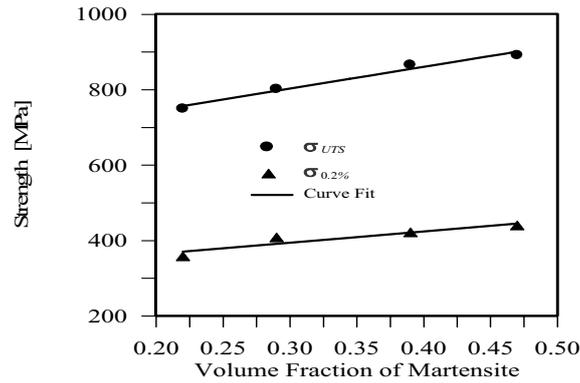
**Figure 6: Variation of strength parameters with the relative amount of martensite**
