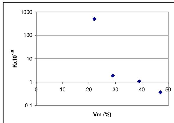
**Figure 9:  $K$  values for different volume fractions of martensite,  $V_m$**
