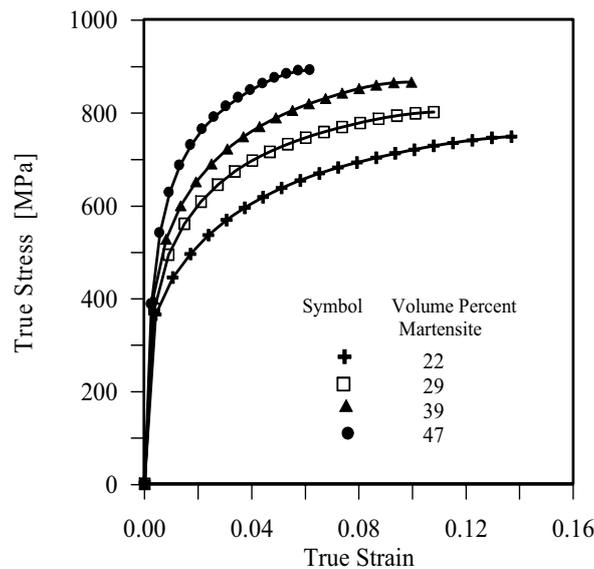
**Figure 5: True stresses True Strain for various volume fraction of martensite**
