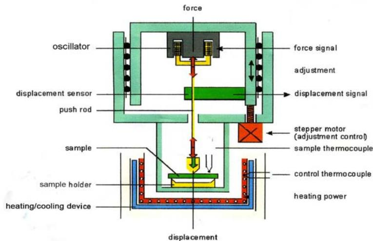
**Figure 1: A diagram of the DMA instrument used in this work [after ref. 7]**
