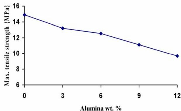
**Figure 2: Effect of alumina weight % on maximum tensile strength.**
