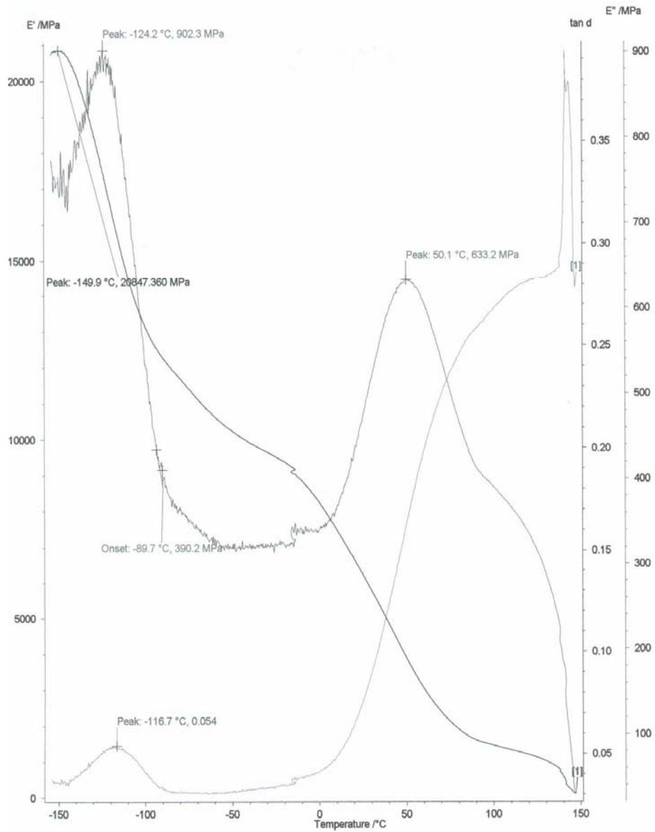
**Figure 4: Variation of  $E'$ ,  $E''$ , and  $\tan \delta$  with temperature for 3 wt% alumina – PE.**
