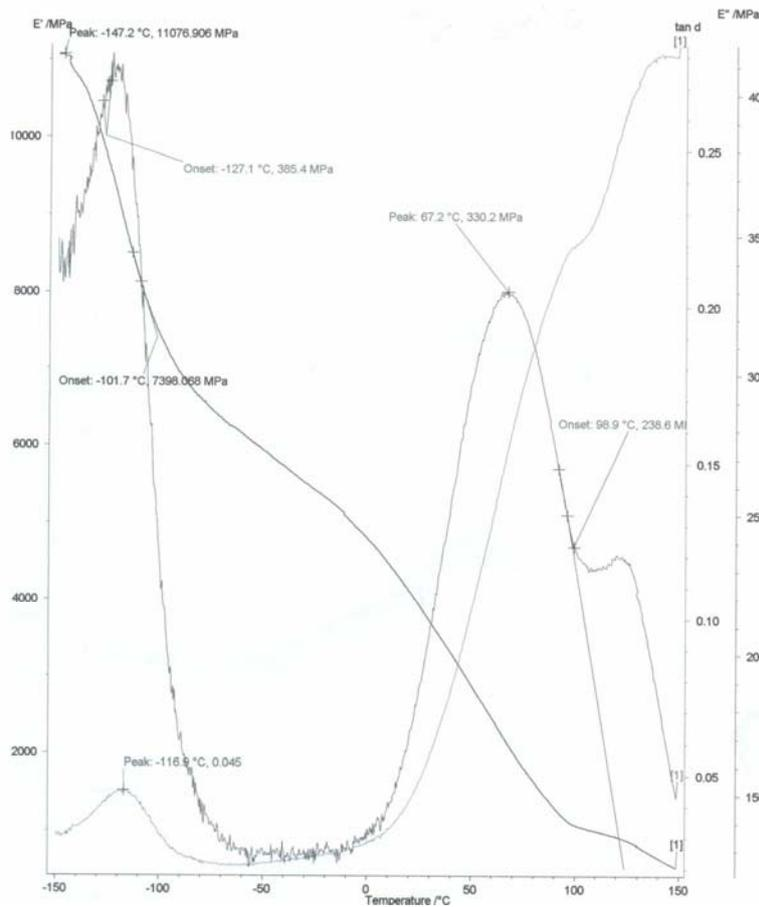
**Figure 5: Variation of  $E'$ ,  $E''$ , and  $\tan \delta$  with temperature for 6 wt% alumina – PE.**
