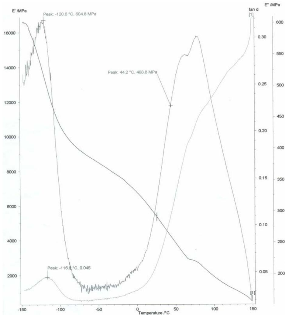
Figure 3: Variation of  $E'$ ,  $E''$ , and  $\tan \delta$  with temperature for pure polyethylene.
