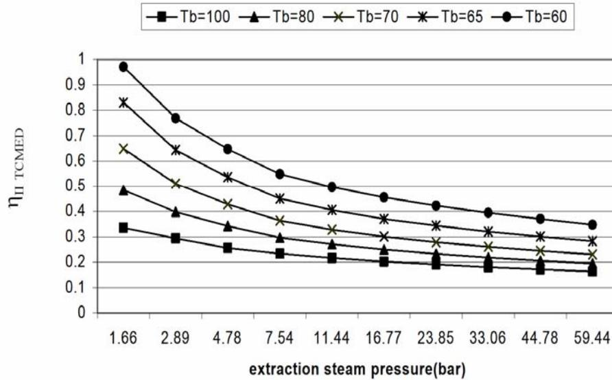
**Figure 6: Effects of the extraction steam pressure and top brine temperature on the partial effectiveness of thermal coupling  $\eta_{II\_TCMED}$**
