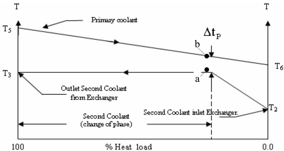
**Figure 4: steam generator temperatures distribution with heat load' %'**
