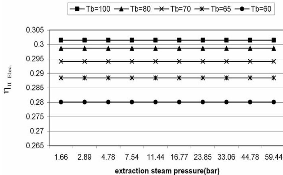
**Figure 7: Effects of the extraction steam pressure and top brine temperature on the partial effectiveness of electricity production  $\eta_{II\_Elec.}$**
