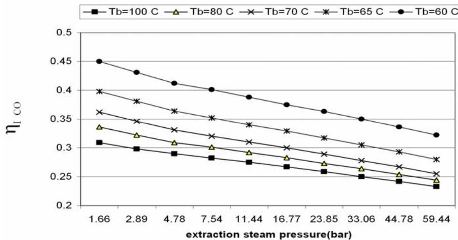
**Figure 5: Effects of the extraction steam pressure and top brine temperature on the  $\eta_{I CO}$**
