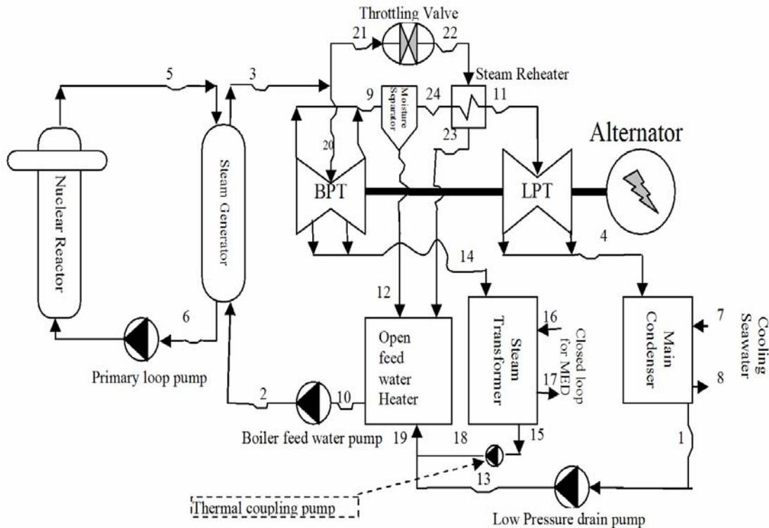
**Figure 2: Diagram of nuclear power plant coupled with desalination plant (MED)**
