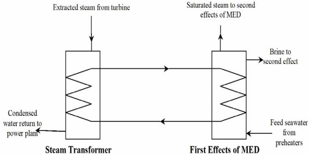
**Figure 3: Schematic diagram shows the circulating loop between steam transformer and first effects of MED plant.**
