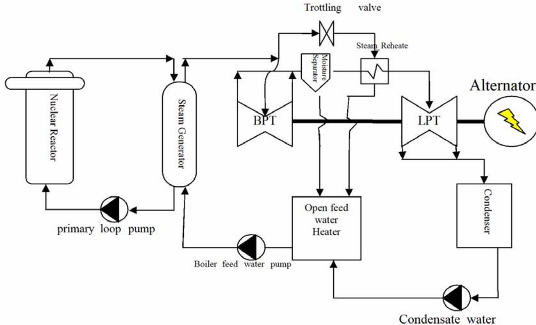
**Figure 1: Typical nuclear powered steam power plant with a pressurized water reactor.**
