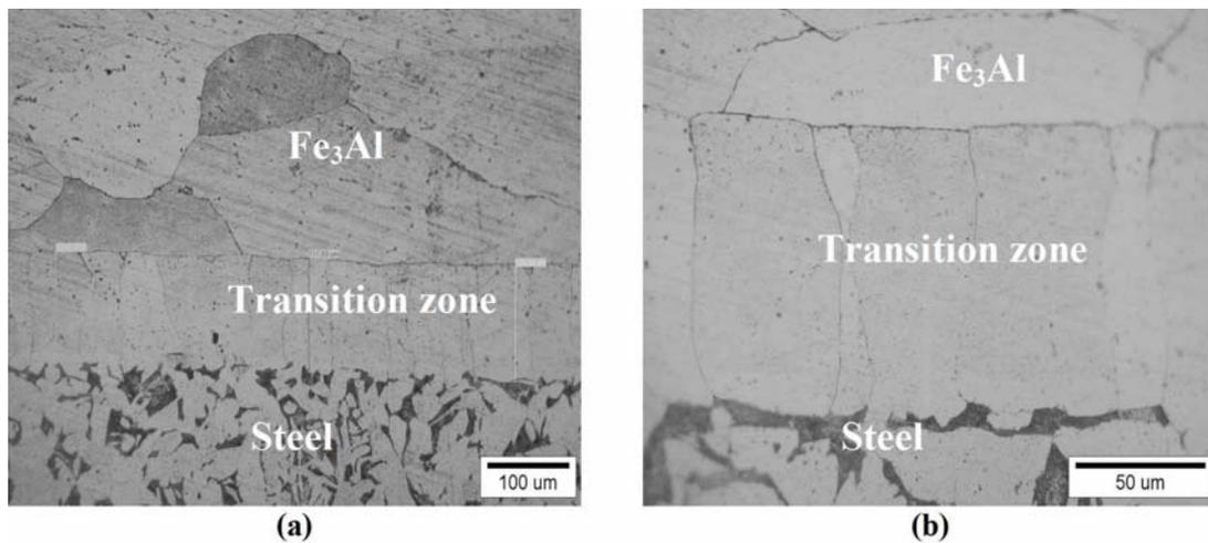
**Figure 10: Optical micrograph of cross-section of Fe<sub>3</sub>Al/steel joint bonded at: T=1100°C; t<sub>b</sub>= 60 min; and P= 10 MPa: (a) The transition zone thickness measurements (119 μm) at x200. (b) x500.**
