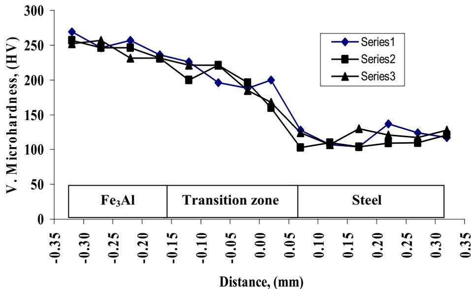
Figure 4: Vickers Microhardness of Fe<sub>3</sub>Al/steel joint bonded at: T=1200 °C; t<sub>b</sub>= 30 min. and P= 10 MPa.
