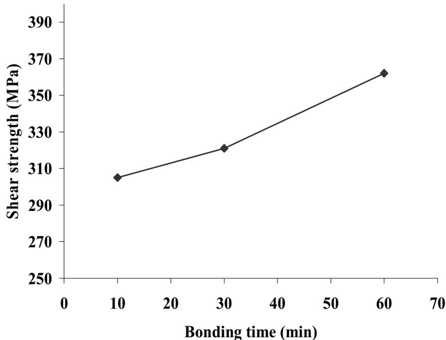
**Figure 2: The effect of holding time on the joint strength of Fe<sub>3</sub>Al/steel joints bonded at: T=1100 °C; P=10 MPa.**
