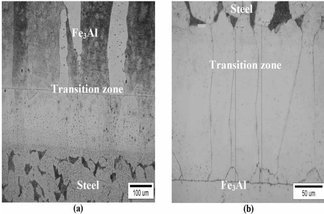
**Figure 7: Optical micrograph of cross-section of Fe<sub>3</sub>Al/steel joint bonded at: T=1100°C; t<sub>b</sub>= 30 min; and P= 10 MPa: (a) x200; (b) The transition zone thickness measurements (159 μm) at x500.**
