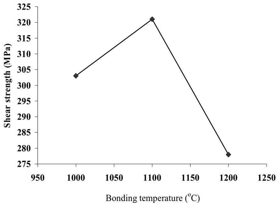
**Figure 1: The temperature dependence of the shear strength of Fe<sub>3</sub>Al/steel joints bonded at: t<sub>b</sub>=30min; P=10 MPa.**
