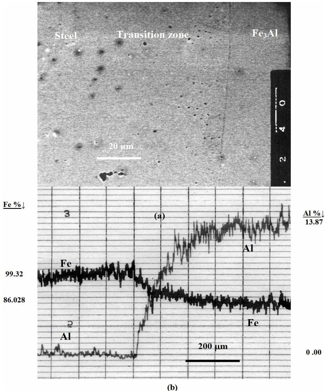
**Figure 11: EPMA line analysis across the Fe<sub>3</sub>Al/steel joint bonded at: T=1100 °C; t<sub>b</sub>= 60 min. and P= 10 MPa: (a) View of the transition zone with line of microanalysis. (b) Distribution of Al and Fe elements across the transition zone.**
