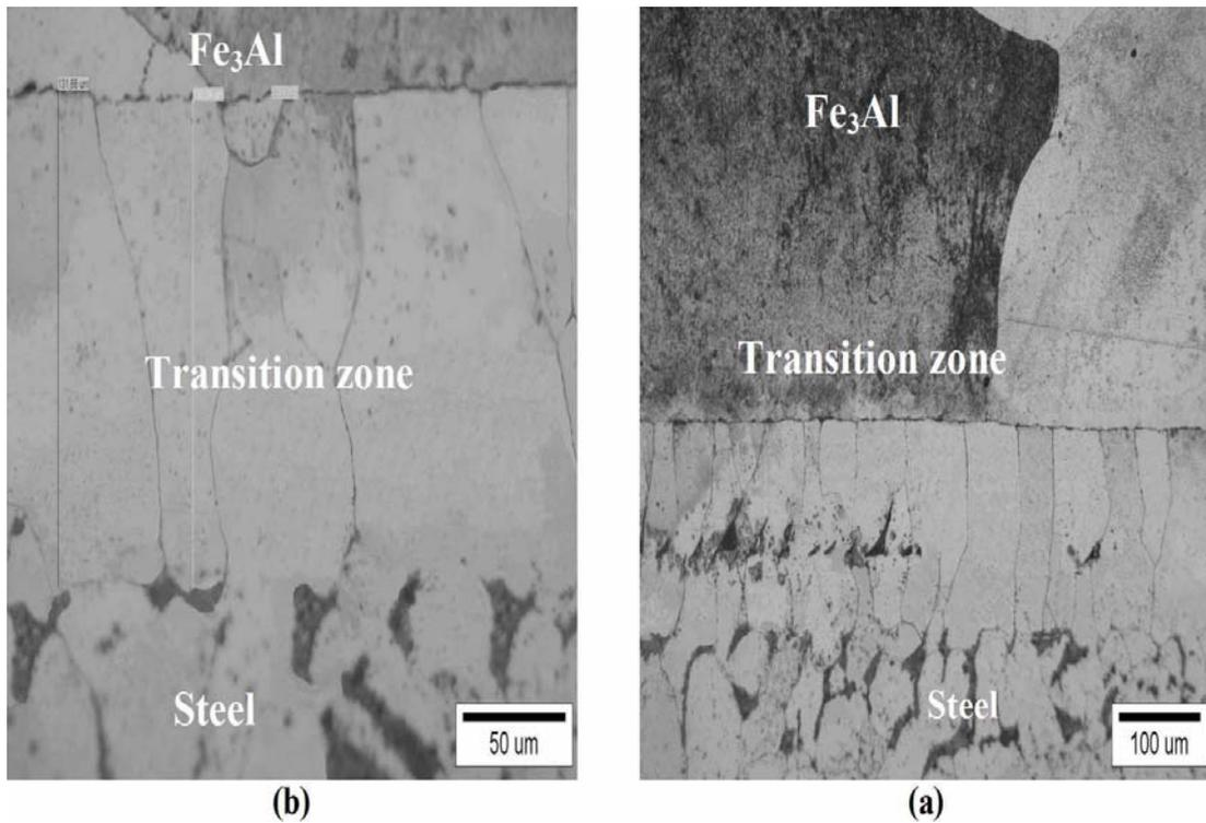
**Figure 8: Optical micrograph of cross-section of Fe<sub>3</sub>Al/steel joint bonded at: T=1200°C; t<sub>b</sub>= 30 min; and P= 10 MPa: (a) x200; (b) The transition zone thickness measurements (136 μm) at x200.**
