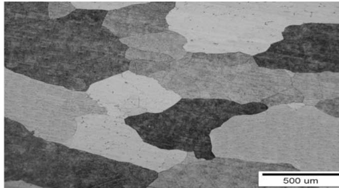
**Figure 5: Optical micrograph of  $\text{Fe}_3\text{Al}$ .**
