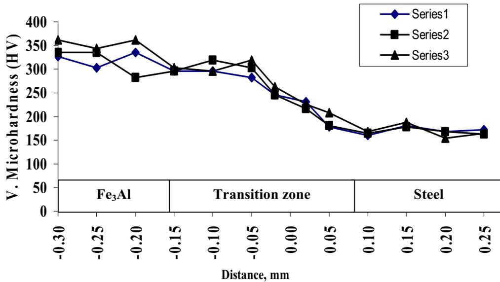
Figure 3: Vickers Microhardness of Fe<sub>3</sub>Al/steel joint bonded at: T=1100 °C; t<sub>b</sub>= 60 min. and P= 10 MPa.
