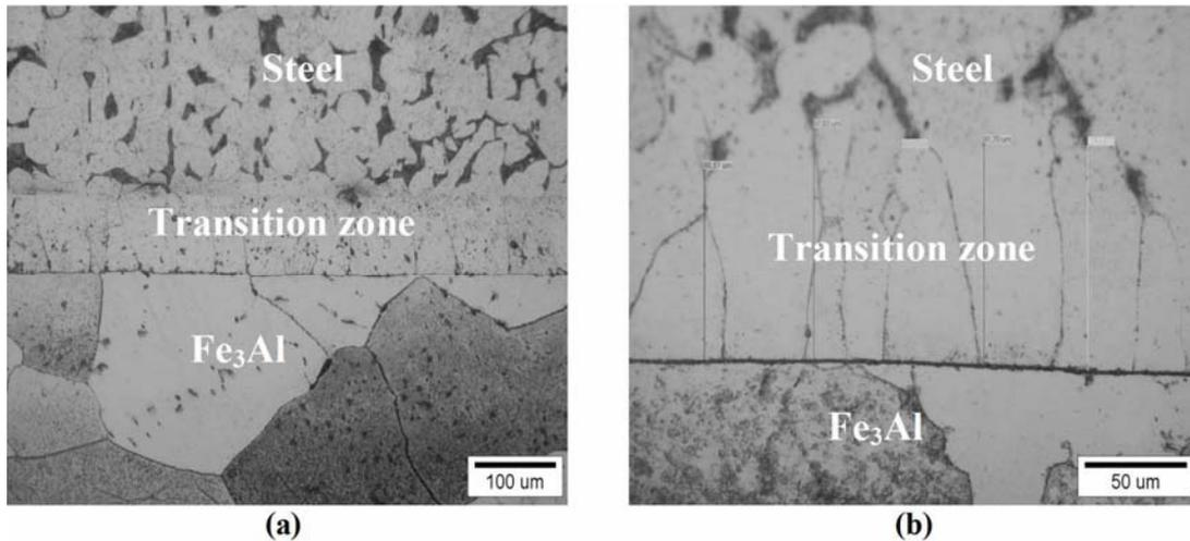
**Figure 9: Optical micrograph of cross-section of Fe<sub>3</sub>Al/steel joint bonded at: T=1100°C; t<sub>b</sub>= 10 min; and P= 10 MPa: (a) x200; (b) The transition zone thickness measurements (98 μm) at x500.**
