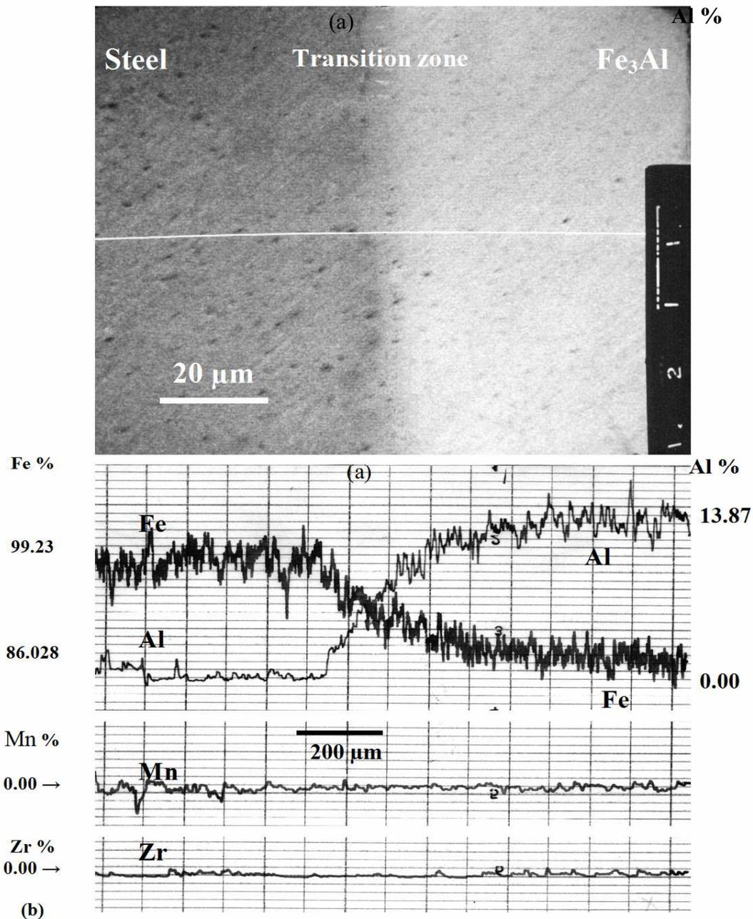
**Figure 12: EPMA line analysis across the Fe<sub>3</sub>Al/steel joint bonded at: T=1200 °C; t<sub>b</sub>= 30 min. and P= 10 MPa: (a) View of the transition zone with line of microanalysis. (b) Distribution of Al, Fe, Mn and Zr elements across the transition zone.**
