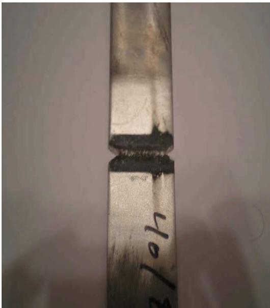
**Figure 1: V notch at joint welding.**
