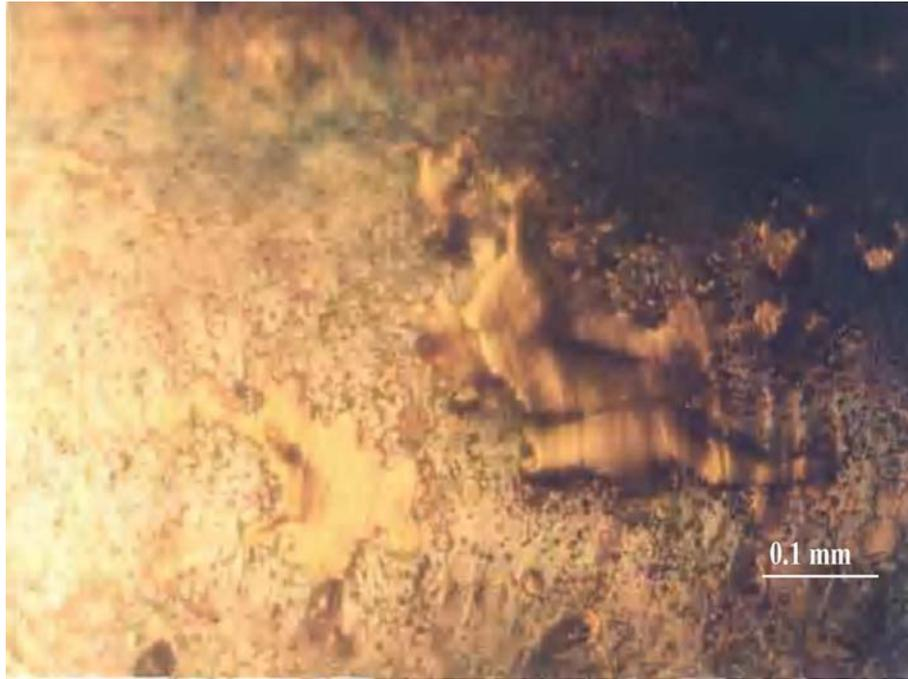
**Figure 4: Grain boundaries separating two grains of the bright layer. These boundaries are oriented perpendicular to the ripple wave fronts.**
