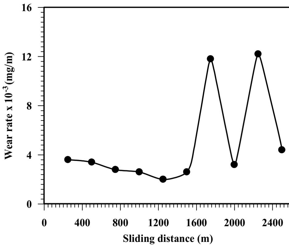
Figure 8: Average wear rates versus sliding distance.
