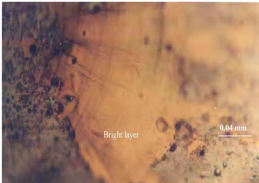
**Figure 3: Bright layer formation at the top of the laser fused tracks.**
