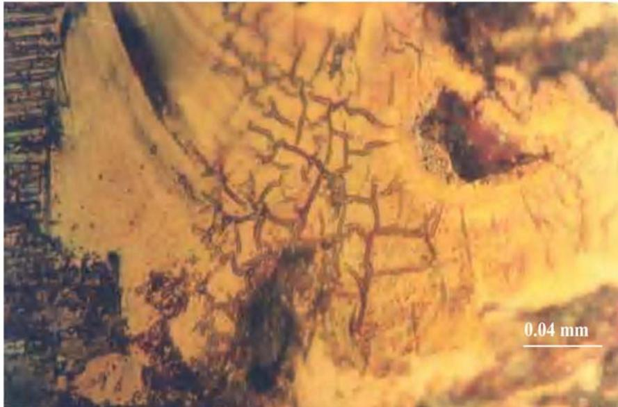
**Figure 6: The thin bright layer at the side of heat affected zone. Note the crack direction.**
