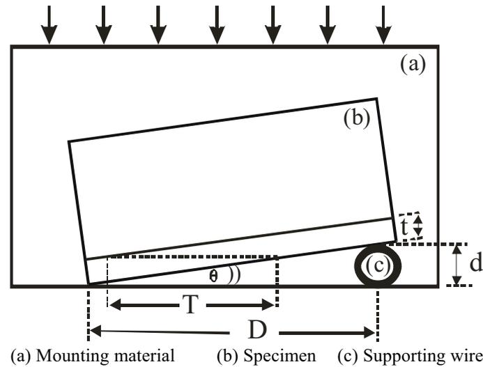
**Figure 1: Oblique mounting of the specimens.**
