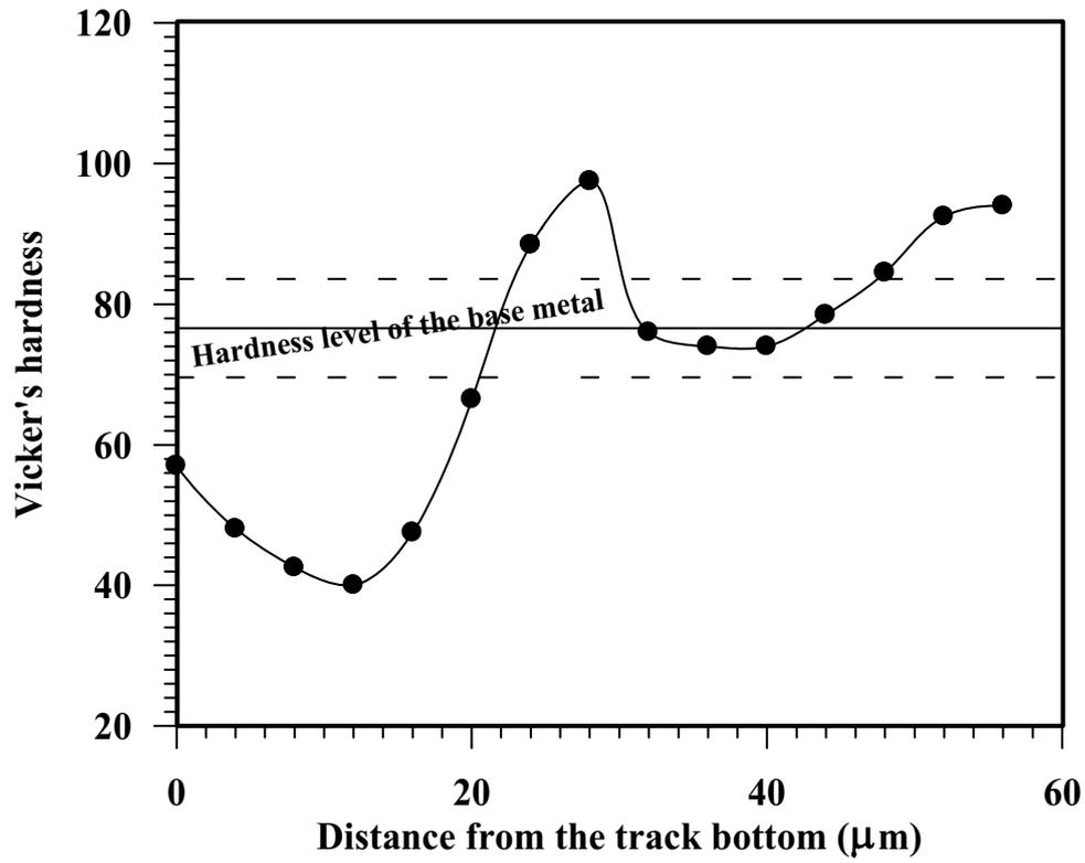
Figure 7: Microhardness through the depth of the tracks.
