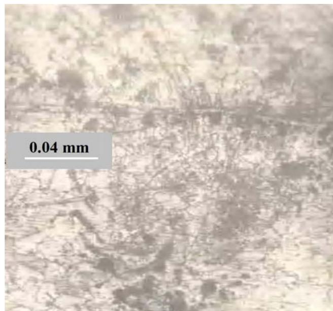
**Figure 9: The effect of the heat treatment on the laser melted tracks. No changes in the microstructure up to 350°C.**
