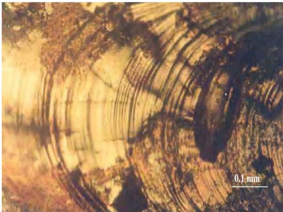
**Figure 5: Sub-grain boundaries outline the cellular growth of the thin surface layers. They are perpendicular to the ripple wave fronts.**
