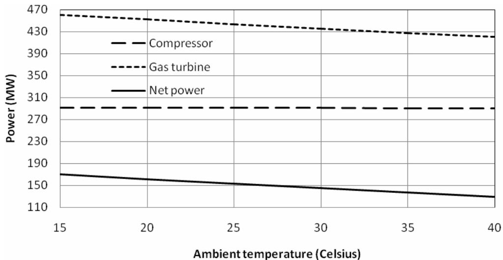
**Figure 3: Effect of ambient temperature on power output**
