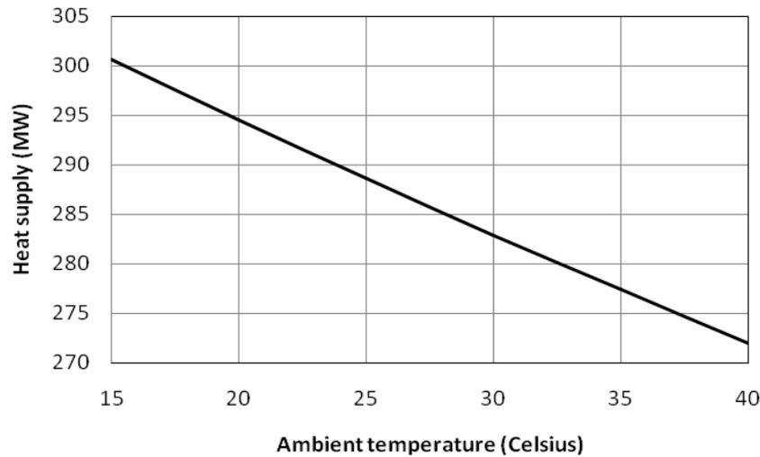
**Figure 4: Effect of ambient temperature on heat supply**
