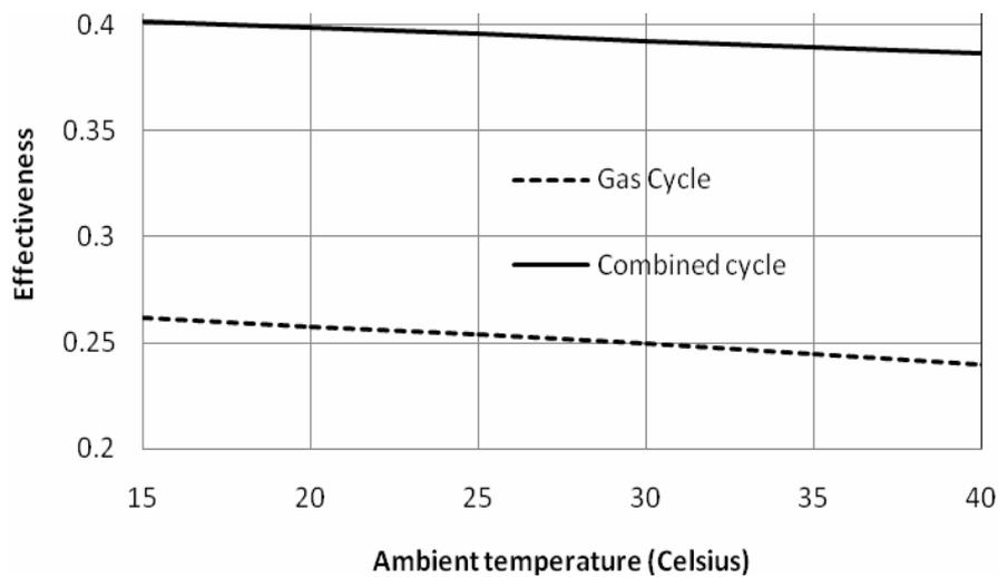
**Figure 9: Effect of ambient temperature on effectiveness**
