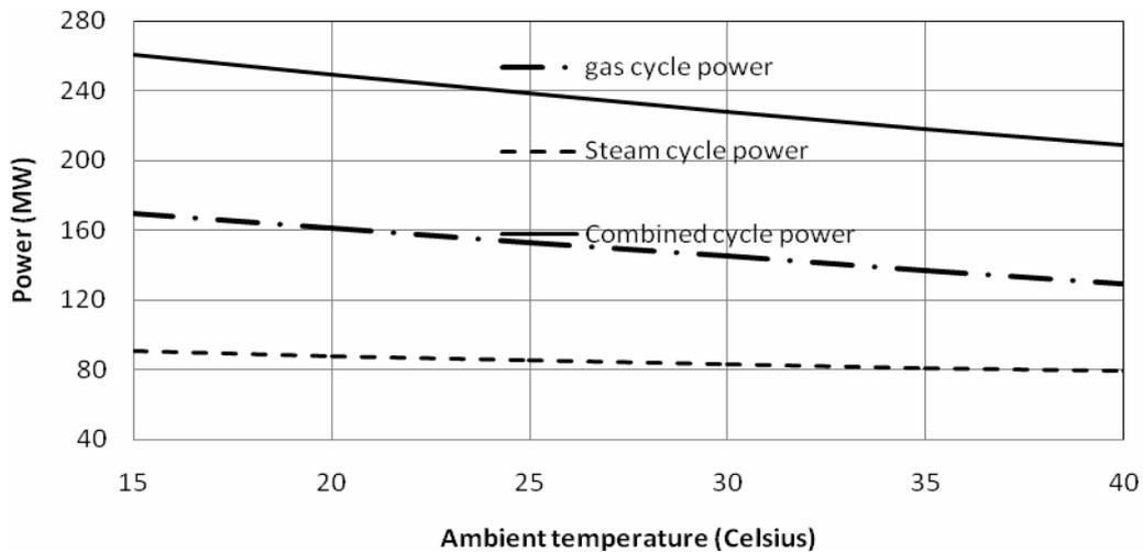
**Figure 5: Effect of ambient temperature on power**
