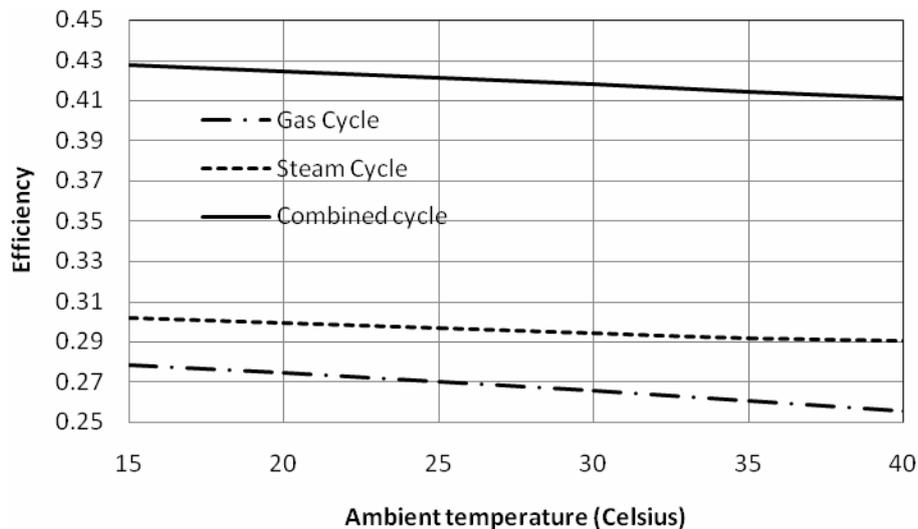
**Figure 7: Effect of ambient temperature on efficiency**
