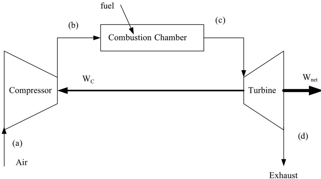
**Figure 1: Schematic of the selected gas turbine power unit**
