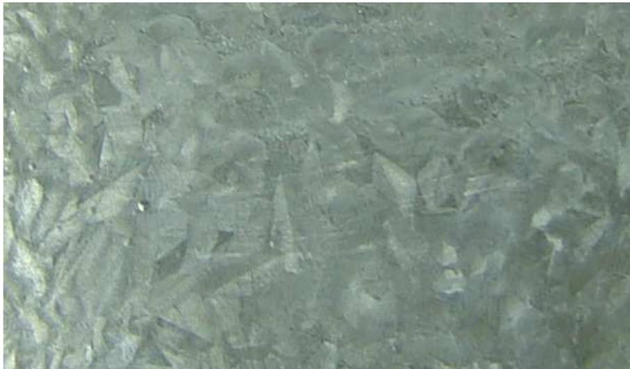
**Figure 4: Surface appearance of galvanized steel obtained at 0.09% wt. Ag, T = 450°C, t = 3 min and v = 3.5 m/min**
