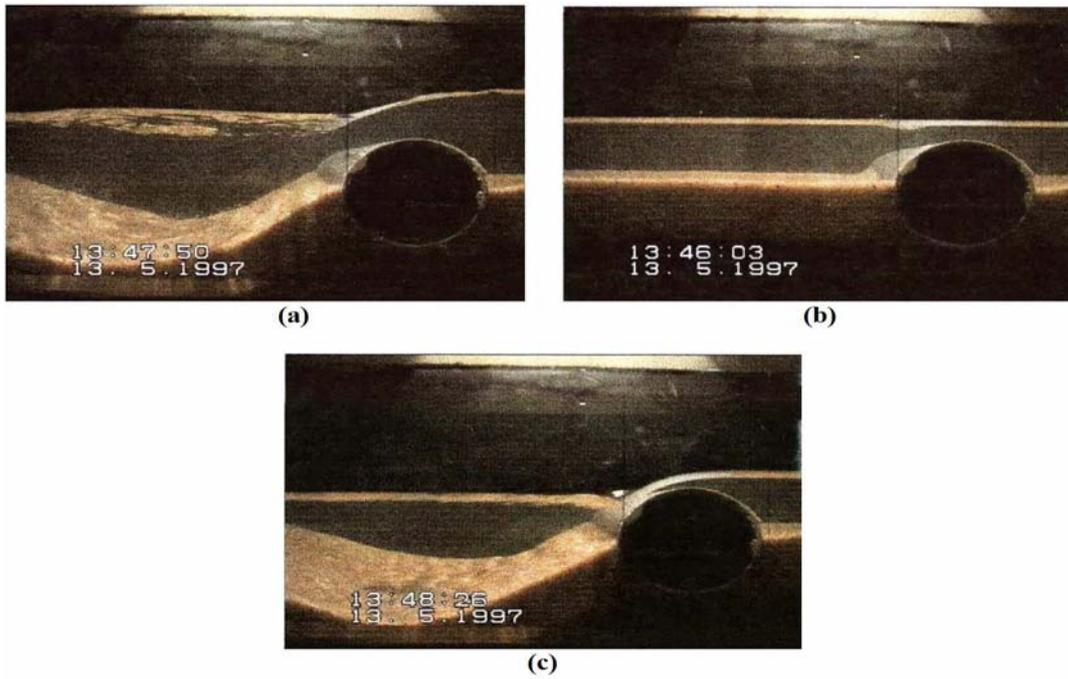
Figure 5: No scour hole in prints a, b, and c for  $h_0/D < 1.0$ , However a scour hole has developed in prints d and e when flow is stopped
