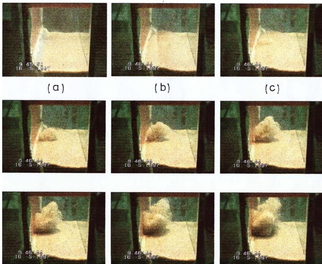
Figure 7: Progress of a tunnel scour due to piping action
