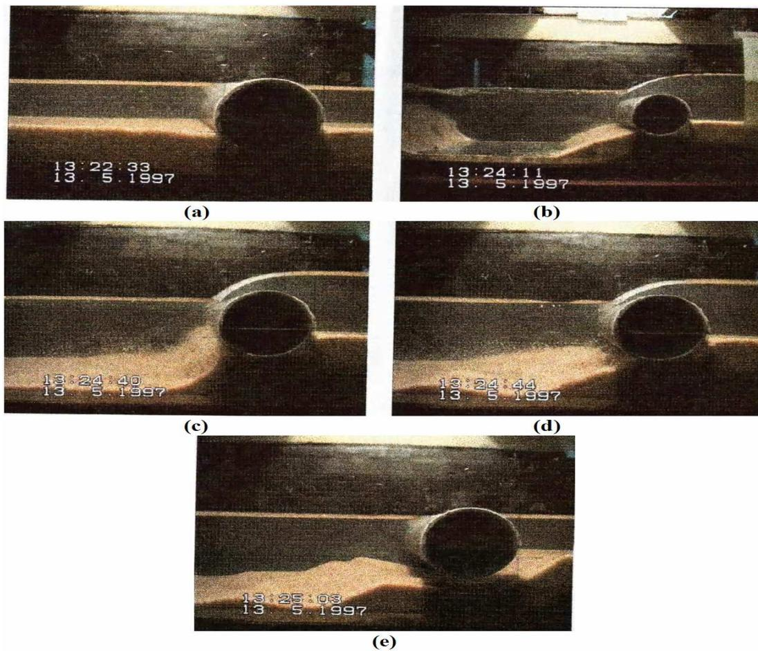
Figure 6: Lack of scour for  $h_0/D < 1.0$  and  $e/D < 0.5$
