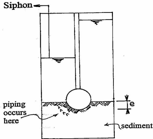
Figure 3: Apparatus for investigating the onset of scour using a static pressure gradient
