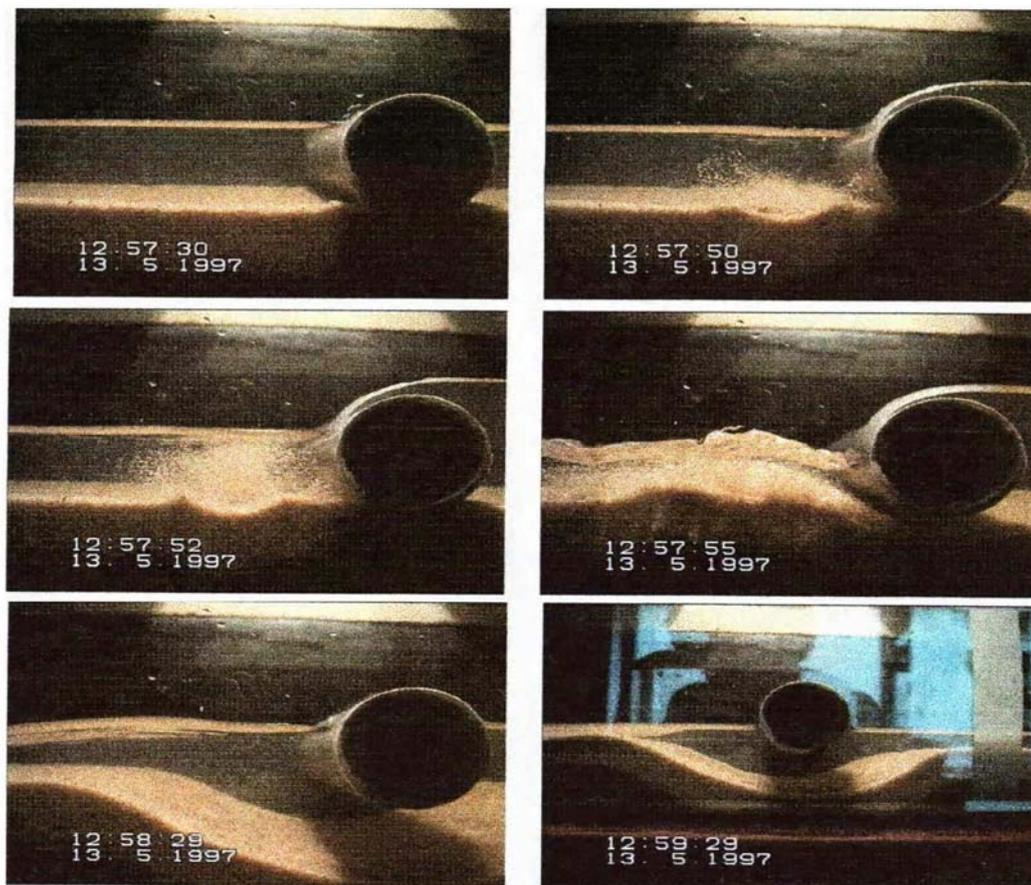
**Figure 4: Progress of a scour hole under a cylinder just resting on sediment**
