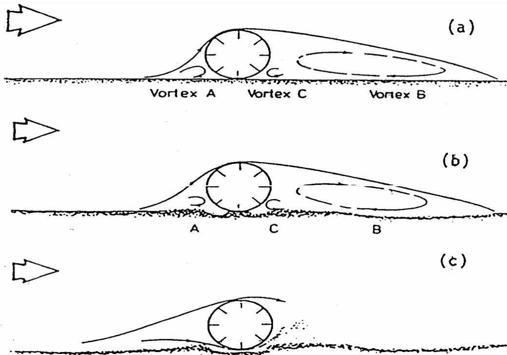
**Figure 1: Three-vortex system and onset of scour, Mao (1988)**
