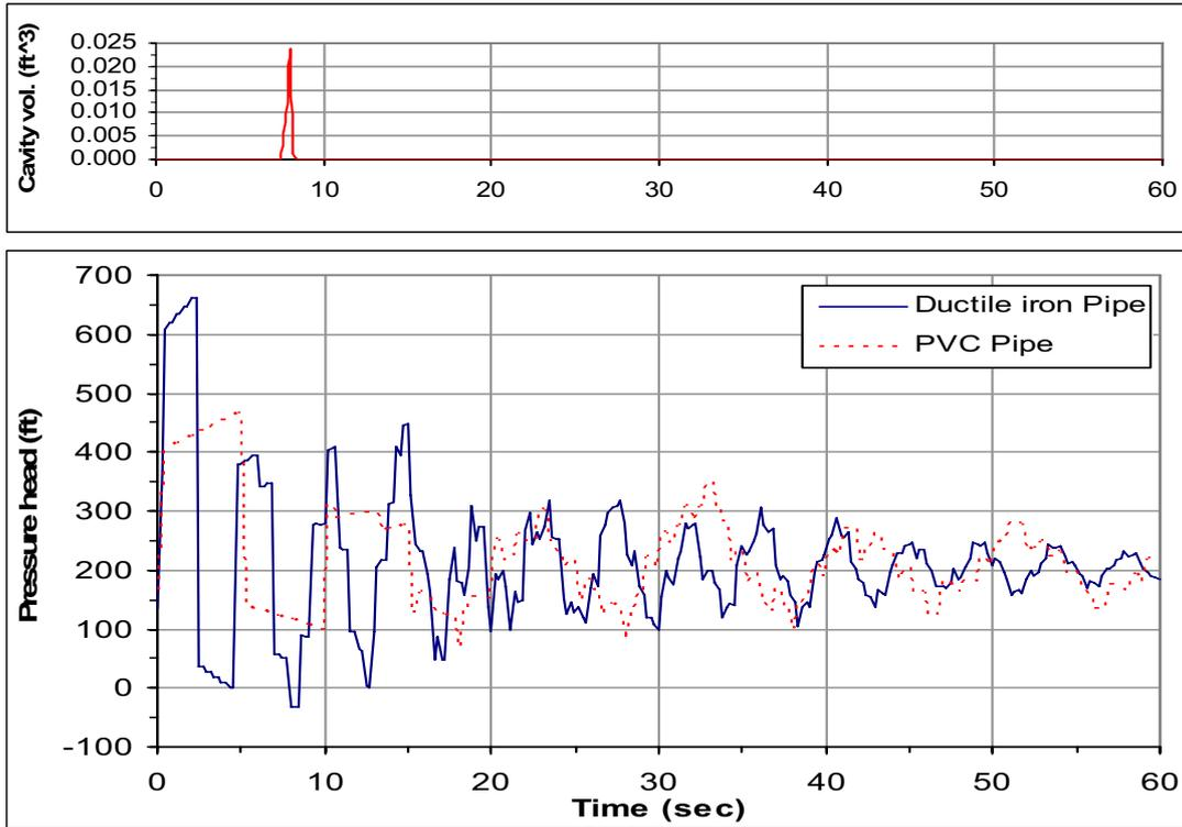
**Figure 8: Effect of using PVC pipes on the local pressure head variations and cavity volume at the end of pipe 5 with closing valve rate (I).**
