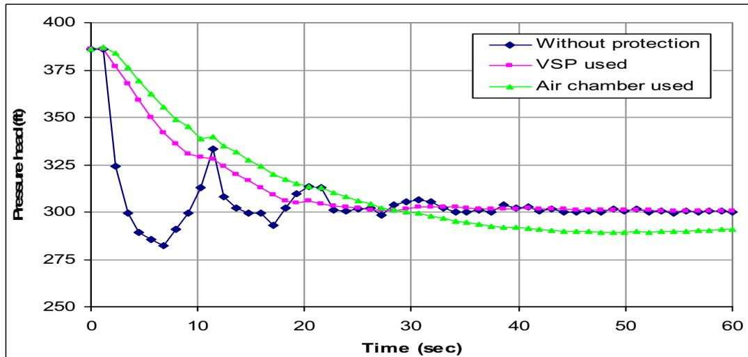
**Figure 10: Effect of protection device on the local transient pressure at downstream end of pipe 6.**
