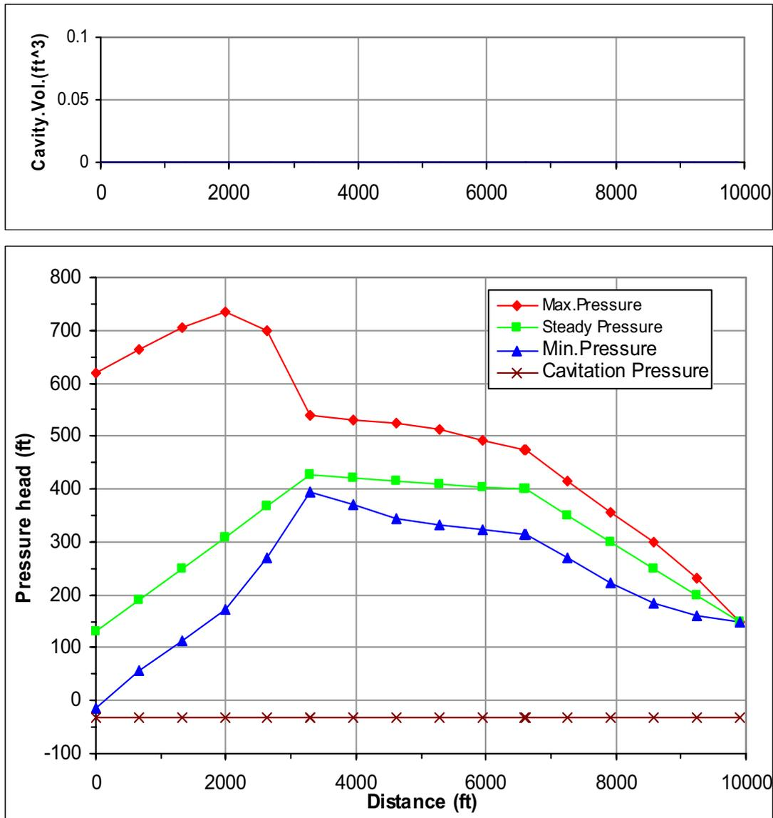
**Figure 6: Pressure and cavity volume along path (TCV-1 → J-3 → J-1 → R-1), due to valve closing rate (III).**
