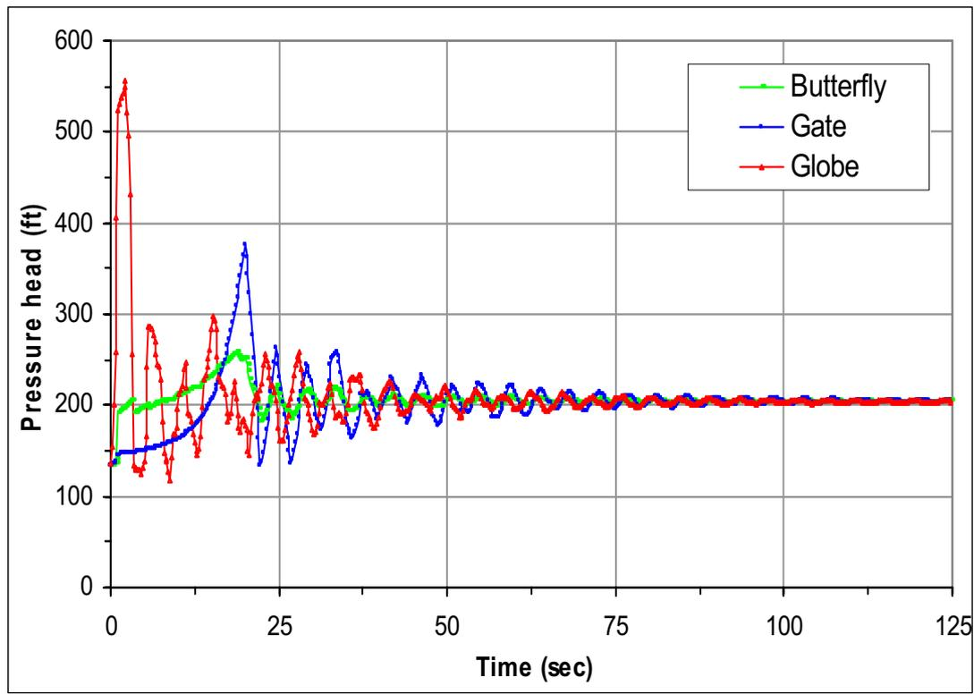
**Figure 7: Effect of valve type on transient pressure head.**
