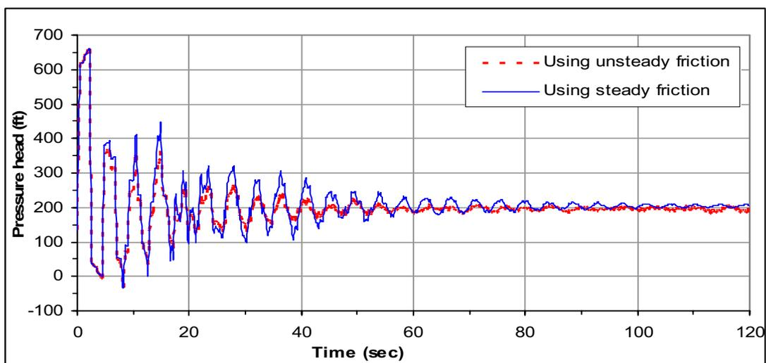
**Figure 11: Effect of friction model used on transient pressure, at upstream of the valve.**
