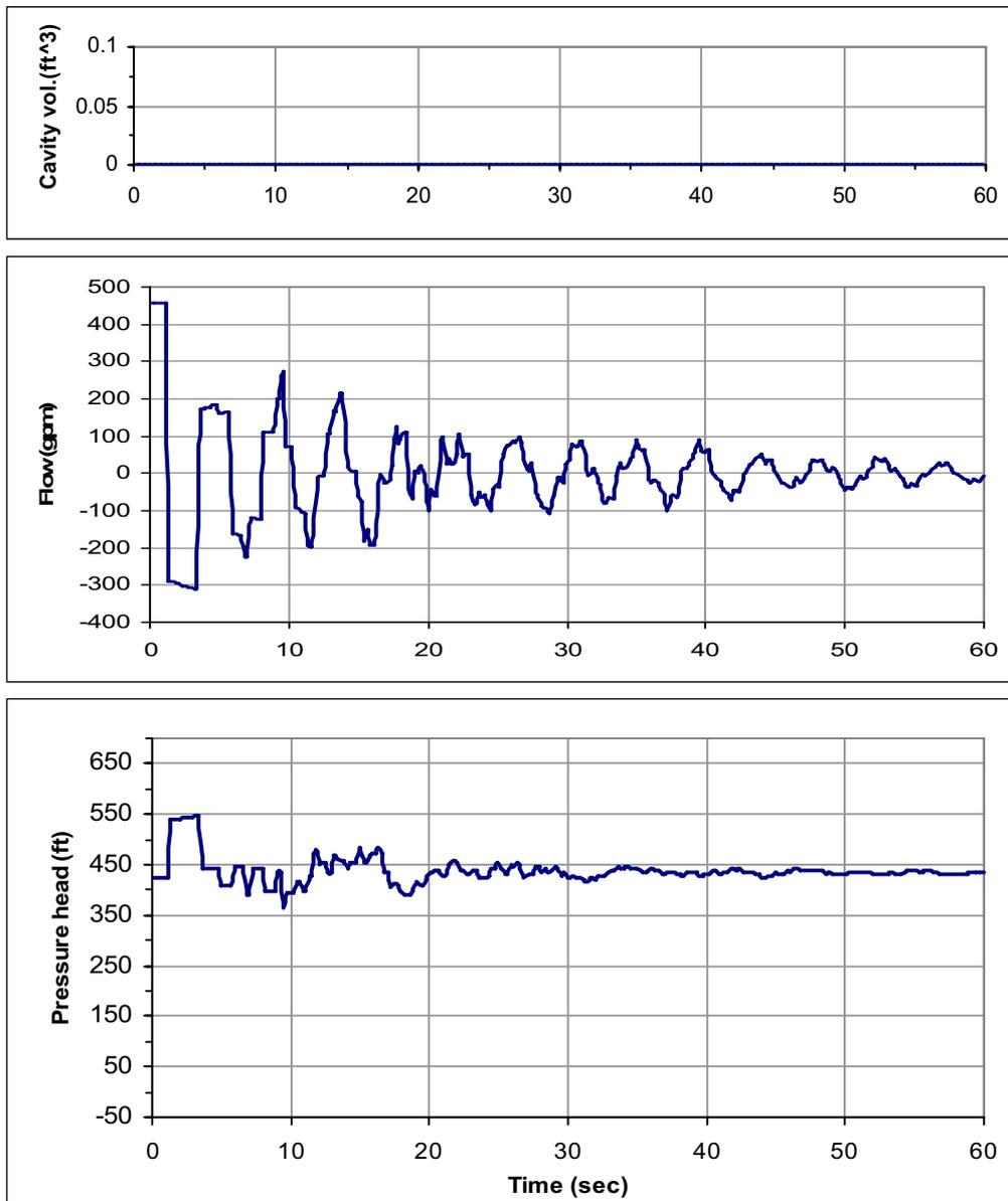
**Figure 3: Transient history (Pressure, Flow & cavity volume) at the upstream end of Pipe 5 (junction 3), using closing rate (I).**
