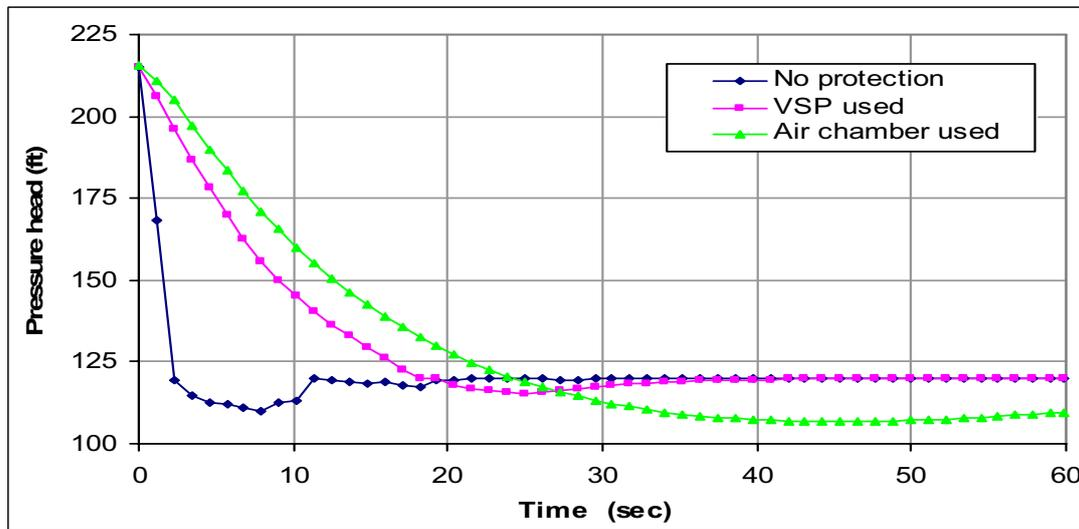
**Figure 9: Effect of protection device on local transient pressure at pump discharge side
