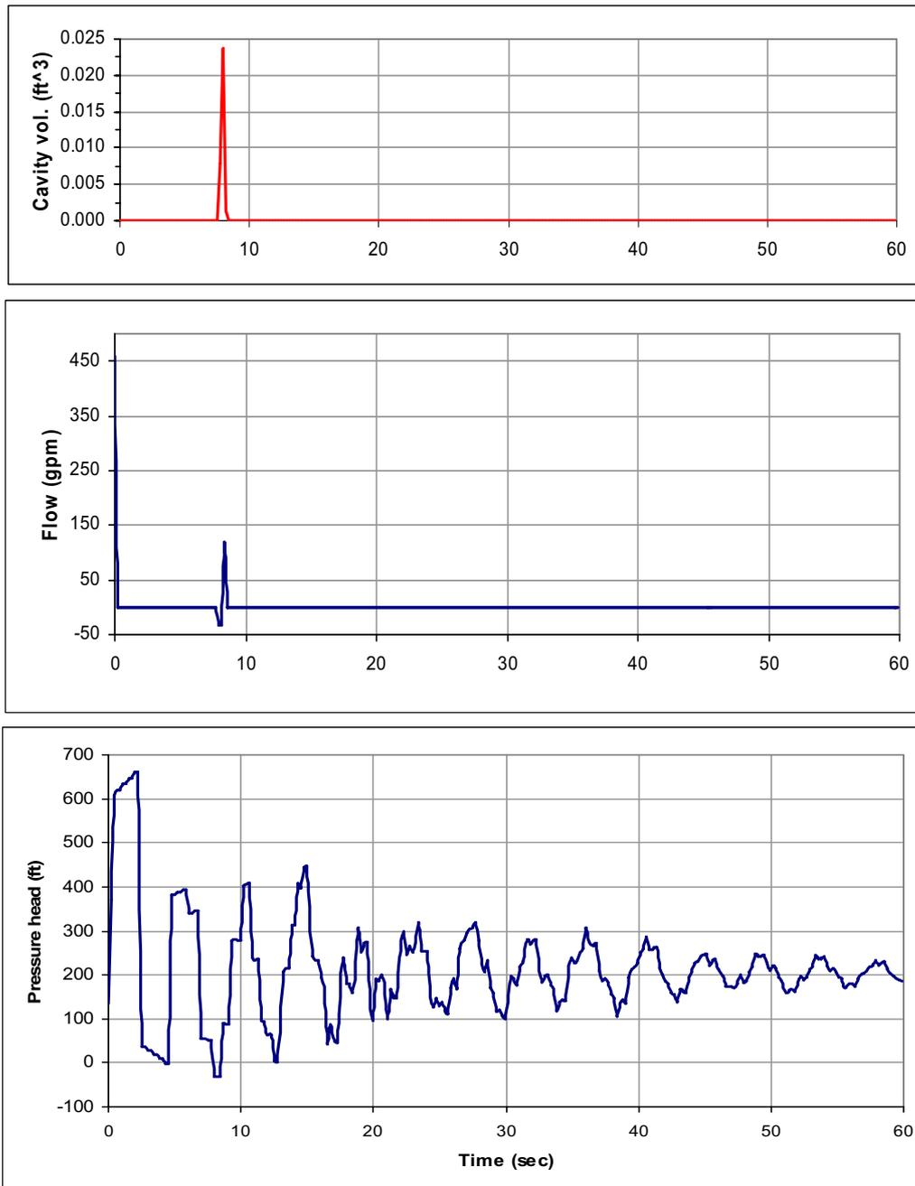
**Figure 2: Transient history (Pressure, Flow & cavity volume) at the upstream end of the valve using closing rate (I).**
