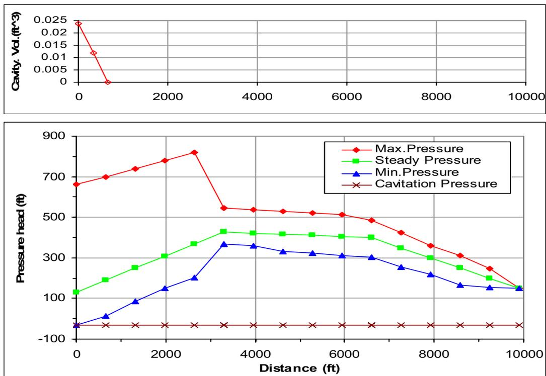
Figure 5: Pressure and cavity volume along path (TCV-1 → J-3 → J-1 → R-1), due to valve closing rate (I)
