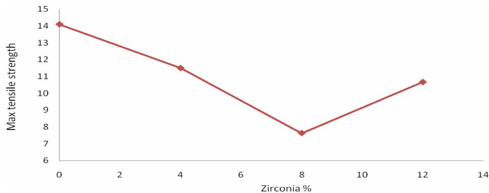
**Figure 2: Effect of zirconia weight (%) on maximum tensile strength**
