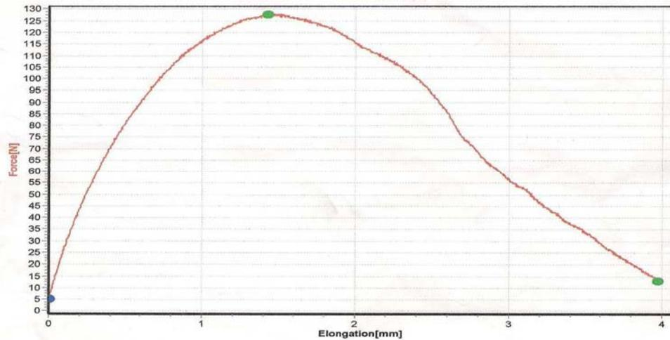
**Figure1: A typical force-elongation curve for one of the composite sheets**
