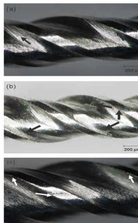
**Figure 1b:** Photomicrographs of K3 instruments (a) K3 file before use (control) showing micro-crack (size 35). (b) K3 file after the tenth use showing chippings (size 25). (c) Chipping and micro-crack after the tenth use (size 40).
