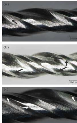
**Figure 1b: Photomicrographs of K3 instruments (a) K3 file before use (control) showing micro-crack (size 35). (b) K3 file after the tenth use showing chippings (size 25). (c) Chipping and micro-crack after the tenth use (size 40).**
