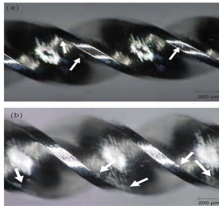
**Figure 1c: Photomicrographs of ProFile instruments. (a) Photomicrograph of unused ProFile instrument (control) showing discontinuity of cutting edge and pitting (size 25). (b) Photomicrograph of ProFile instrument after the tenth use, showing signs of wear on the cutting edge (size 35).**
