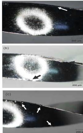
**Figure 1a: Photomicrographs of EndoWave files. (a) EndoWave files before use (control) showing pitting and discontinuity of cutting edge (size 40). (b) Wear of EndoWave file after the tenth use (size 30). (c) Micro-fractures (arrows) after the tenth use (size 25).**
