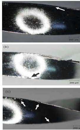
**Figure 1a:** Photomicrographs of EndoWave files. (a) EndoWave files before use (control) showing pitting and discontinuity of cutting edge (size 40). (b) Wear of EndoWave file after the tenth use (size 30). (c) Micro-fractures (arrows) after the tenth use (size 25).
