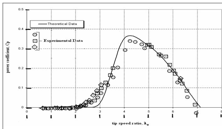
Figure 3: Comparison of computer program results with wind tunnel test results
