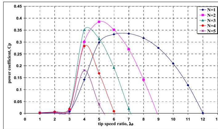
Figure 4: The Effect of Number of Blades on the  $C_p(\lambda_0)$  Curve for Constant  $(C/R)$  of 0.09 and at  $(H/R) = 1$
