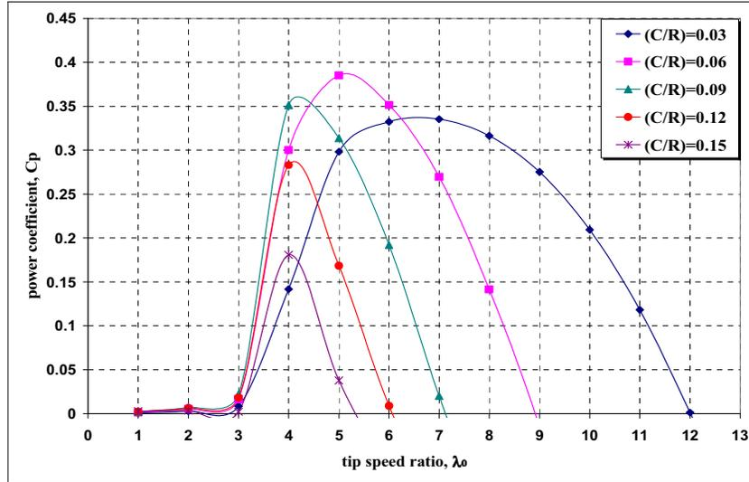
Figure 5: Chord to Radius Ratio Effect on  $C_p(\lambda_0)$  Curve for Constant Number of Blades of 3 and at  $(H/R) = 1$ .
