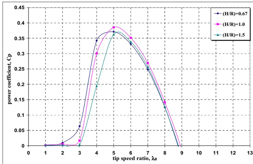
Figure 7: Height to Diameter Ratio Effect on  $C_p(\lambda_0)$  Curve for  $(NC/R) = 0.18$ .
