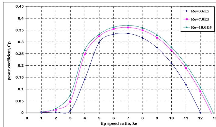
Figure 9: Reynolds Number Effect on  $C_p(\lambda_0)$  Curve for (H/R) of 1.0 and (NC/R) = 0.09
