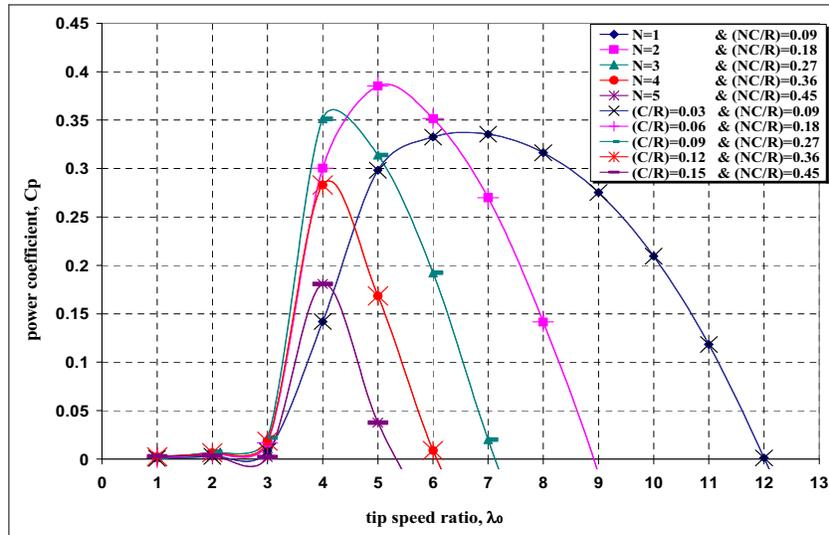
Figure 6: Coincidence of  $C_p(\lambda_0)$  Curves for Pairs of Rotor Configurations with  $(H/R)=1$  and Having Different  $N$  or  $(C/R)$  but Identical  $(NC/R)$ .
