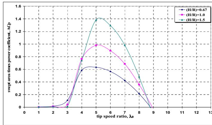
Figure 8: Variation of (ACp) with Tip Speed Ratio for Different (H/R) Values but Constant (NC/R) of 0.18
