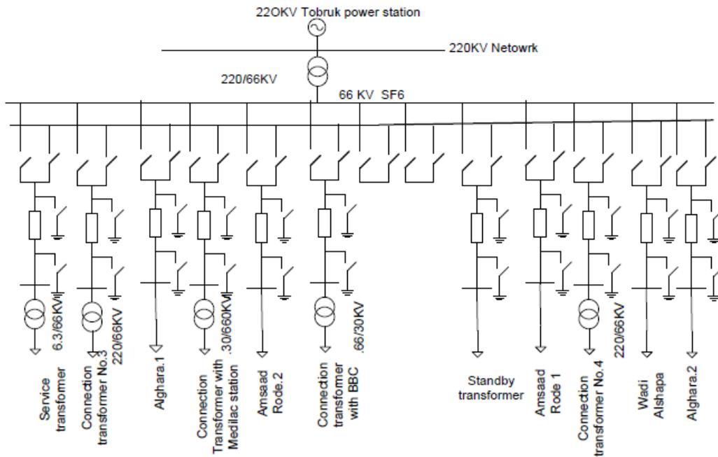
**Figure 3: Tobruk 66kV Network (bus bars, transformers and feeders).**
