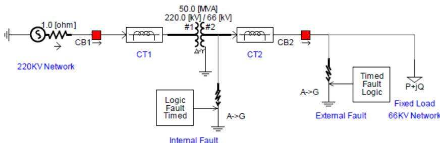
**Figure 7: Internal Fault and External Fault Location**
