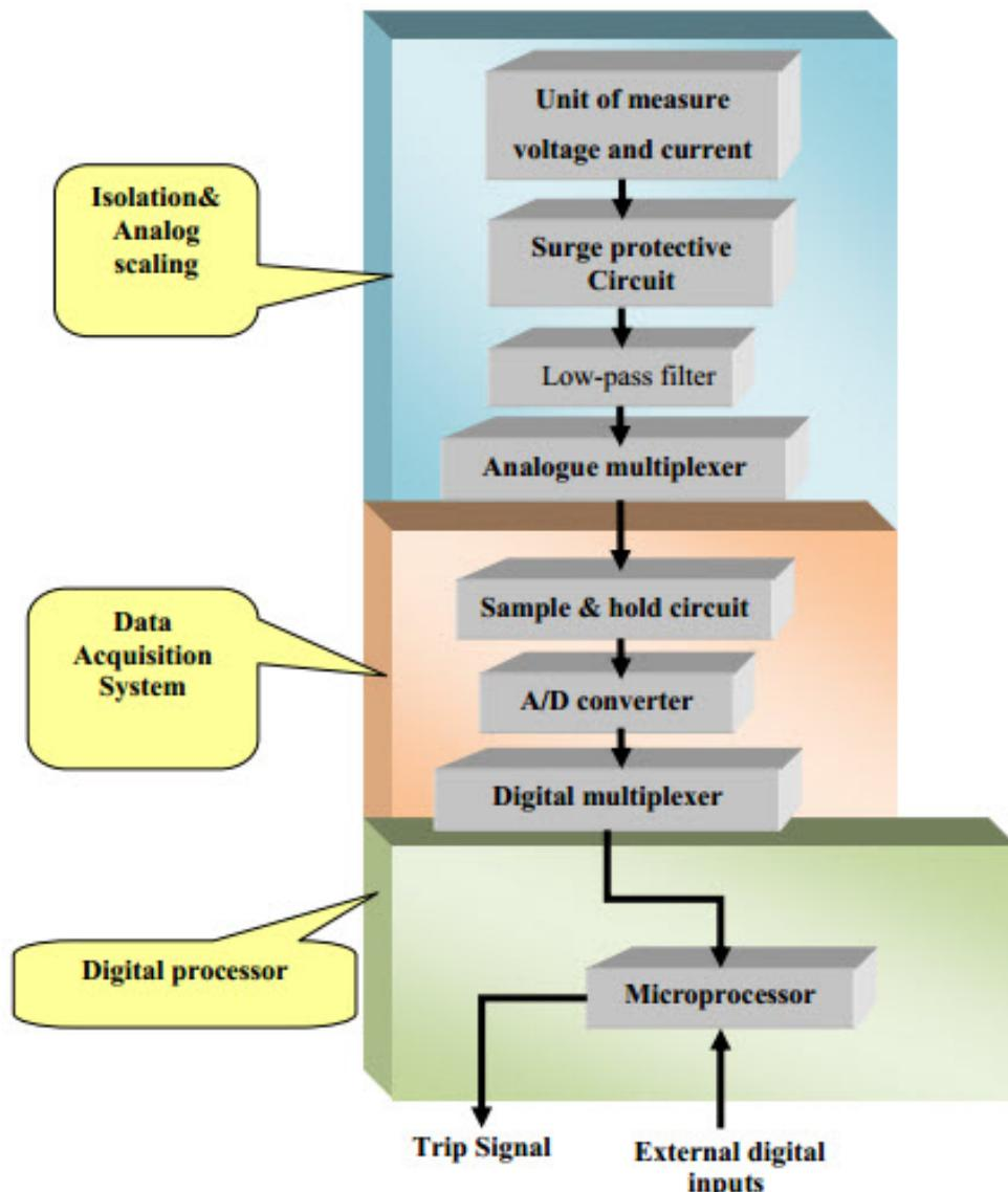
Figure 1: Generalized digital relay structure
