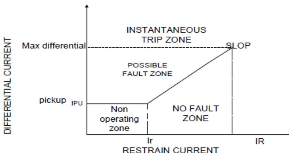
Figure 2: The characteristic of a percentage differential protection
