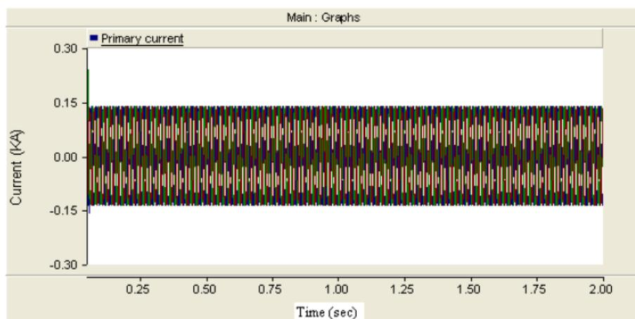
**Figure 9: Primary current during normal operation**
