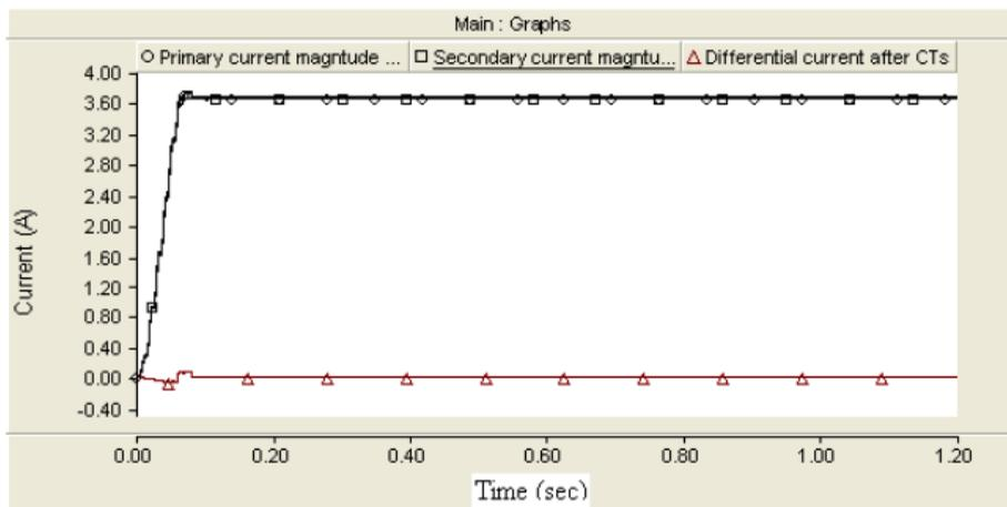
**Figure 11: Primary, secondary and differential currents at normal operation.**
