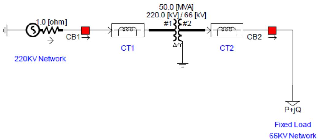
**Figure 4: Single line Diagram of the Simulation Model**
