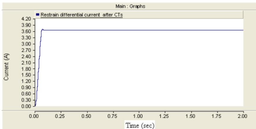
**Figure 12: Restrain current from CT secondary currents**
