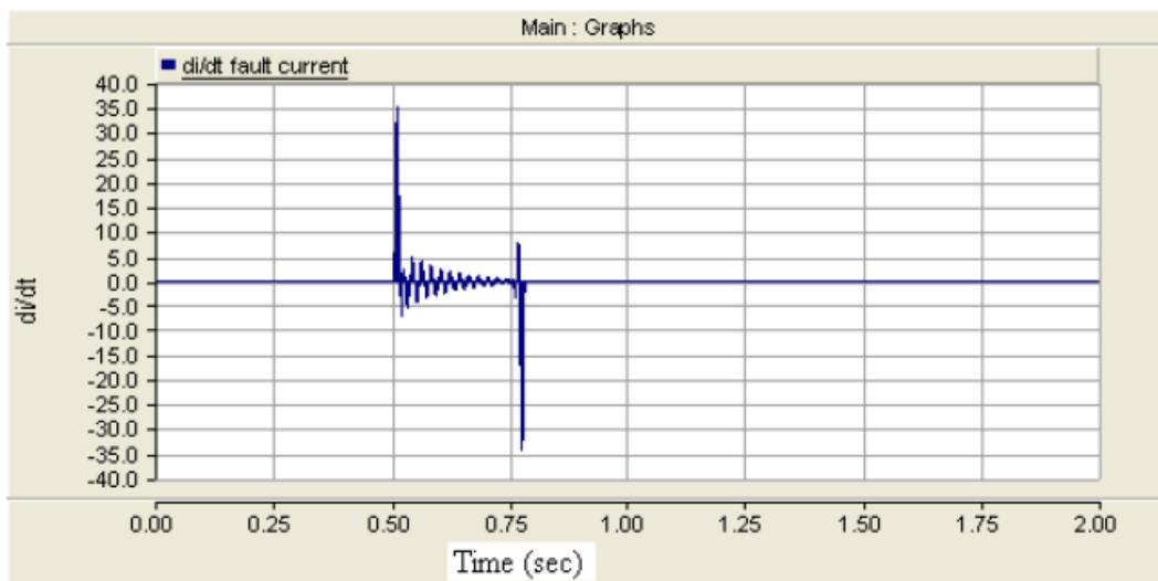
**Figure 14: Derivative of internal fault current**
