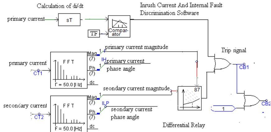
**Figure.6: The digital relay in PSCAD**
