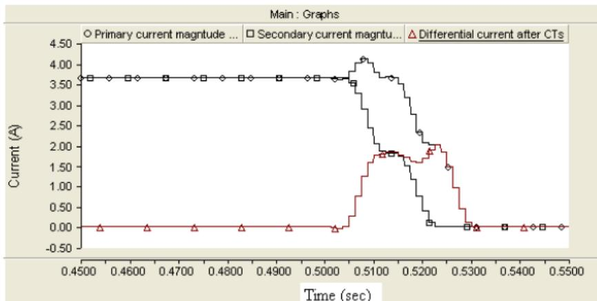
Figure 18: Primary, secondary and differential currents during internal fault.
