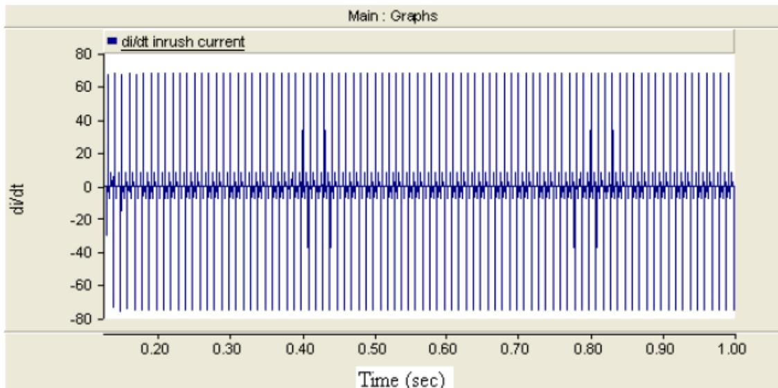
**Figure 15: Derivative of inrush current**
