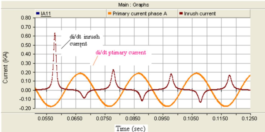
**Figure 13: Inrush current and primary current waveform**
