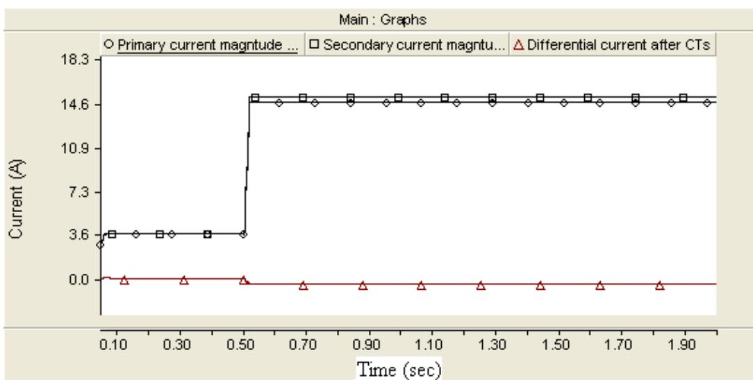
**Figure 20: Primary, secondary and differential currents during external fault**
