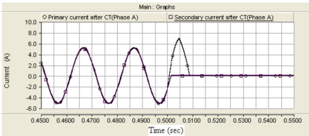
Figure 17: The output CTs of the primary and secondary current waves of phase A
