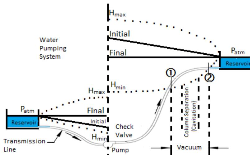
Figure 5: Case study for a pumping system suffers from a pump failure [6].
