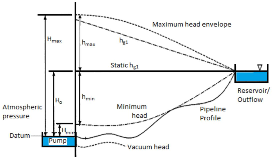
Figure 2: Pipeline profile with definitions of pressure heads [6].
