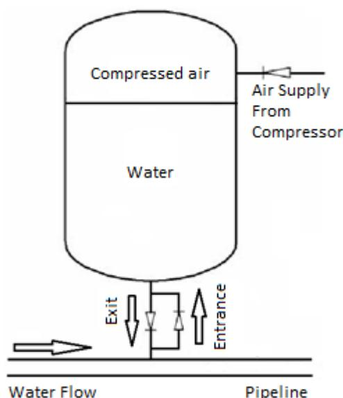
Figure 1: Schematic of air vessel
