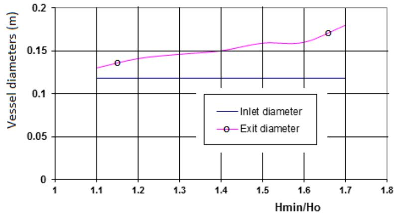
**Figure 20: Inlet and outlet diameters of the air vessel with minimum head ratio.**
