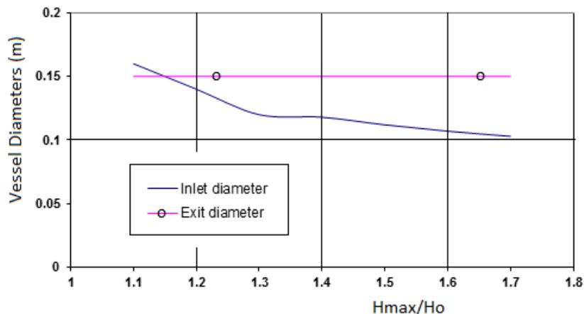
**Figure 21: Inlet and outlet diameters of the air vessel with maximum head ratio.**
