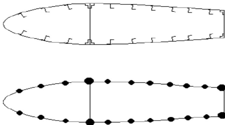
**Figure 2: Original and Idealized wing sections, [1]**
