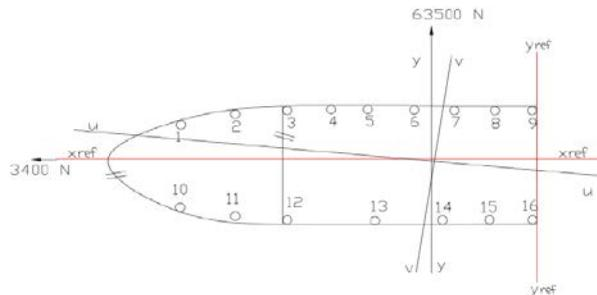
Figure 14: Idealized unsymmetrical double cell wing box, [3, 6-7].
