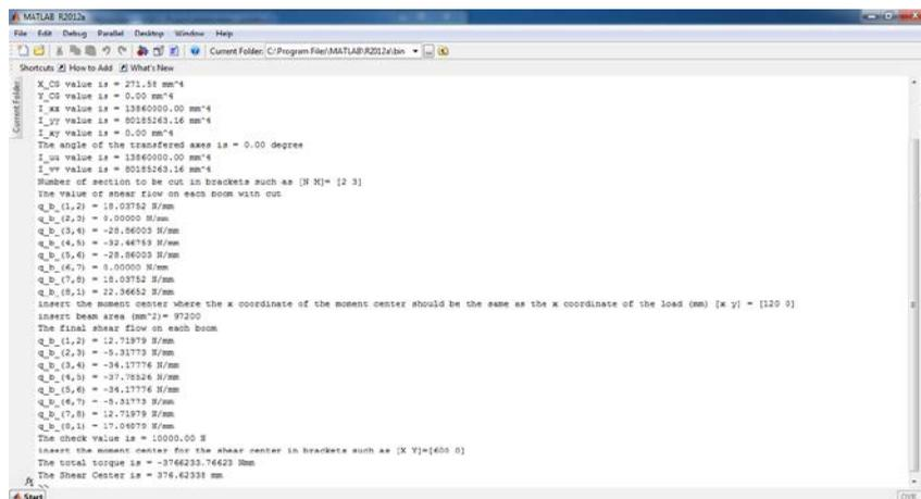
Figure 13: Developed program results, Matlab of the single cell wing box.
