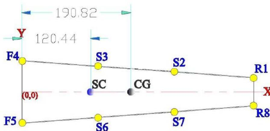
Figure 10: Theoretical Centre of gravity and shear centre of fabricated single cell.
