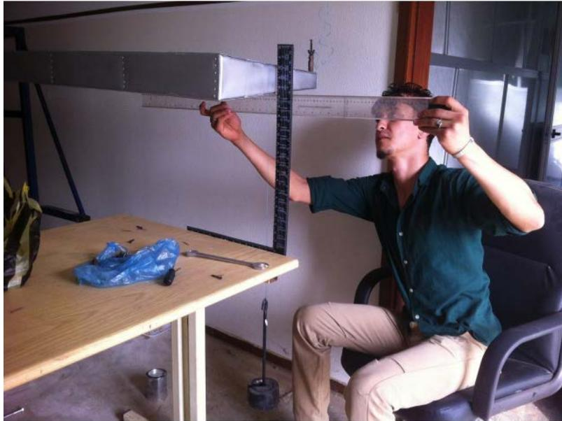
**Figure 11: Deflection tests of the fabricated single cell wing box.**
