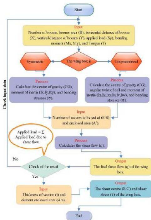
Figure 4: Flow chart of the program for the single cell wing box
