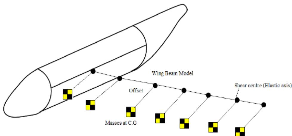
**Figure 1: Simplified wing beam with lumped masses**
