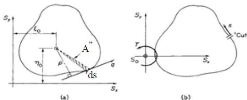
Figure 3: (a) determination of  $q_{s,0}$ , (b) equivalent loading on open section beam, [1].
