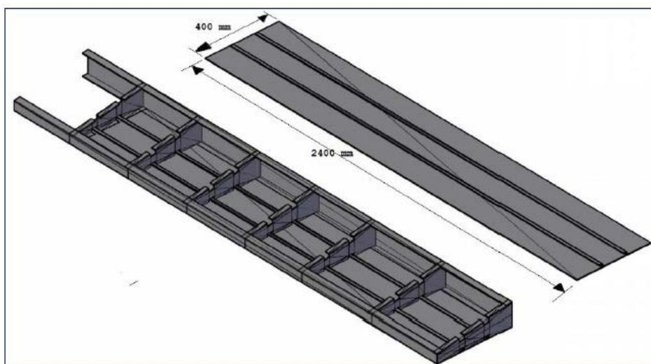
**Figure 6: General view of the wing box using AutoCAD program.**
