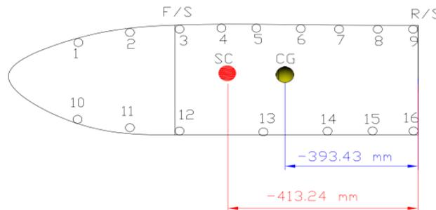
Figure 17: Centre of gravity and shear centre for the double cell wing box.
