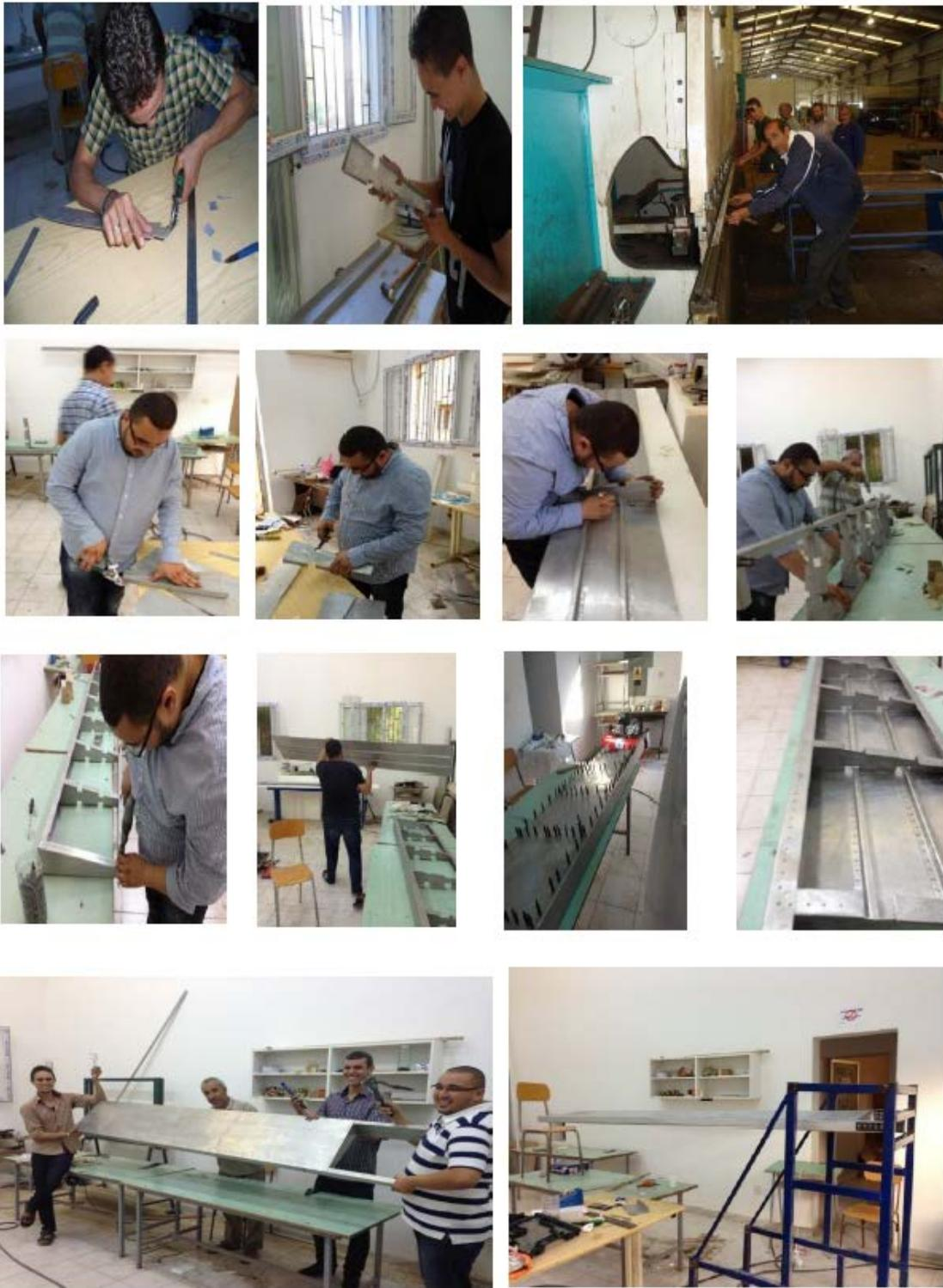
**Figure 7: Fabrication steps of the single cell wing box.**
