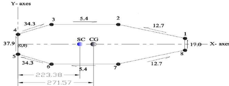
Figure 12: Section Properties and final shear flow of the single cell wing box, [1].
