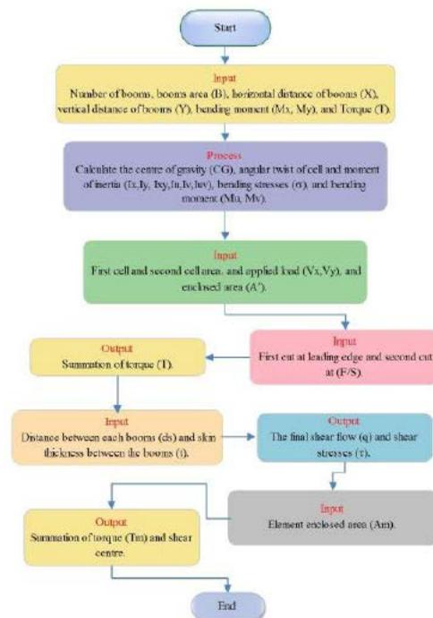
Figure 5: Flow chart of the for the double cell wing box
