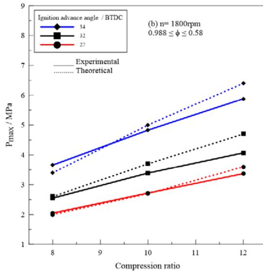
**Figure 2b: Effect of compression ratio on Maximum cylinder gas pressure (1800 rpm).**
