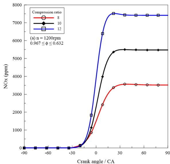
**Figure 5a: Effect of compression ratio on  $NO_x$  (1200rpm)**
