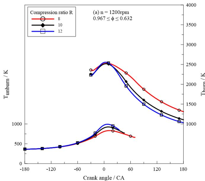
**Figure 4a: Effect of compression ratio on  $T_{\text{burn}}$  and  $T_{\text{unburn}}$  (1200 rpm).**
