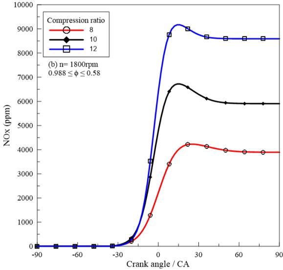
Figure 5b: Effect of compression ratio on  $NO_x$  (1800rpm)
