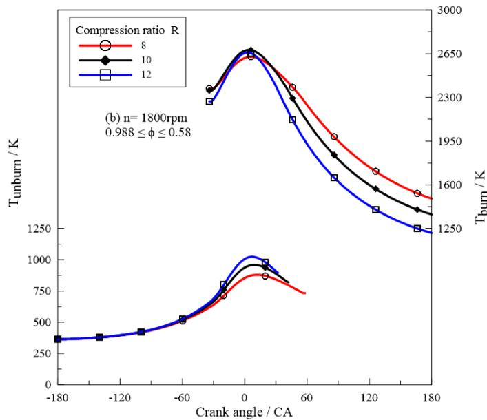
**Figure 4b: Effect of compression ratio on  $T_{burn}$  and  $T_{unburn}$  (1800 rpm).**
