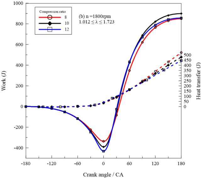
Figure 6: Effect of compression ratio on work and Heat transfer (1800rpm)
