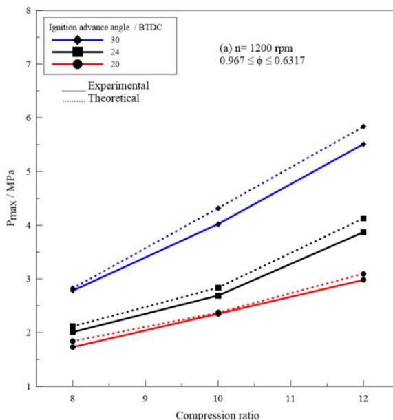
Figure 2a: Effect of compression ratio on Maximum cylinder gas pressure (1200 rpm).
