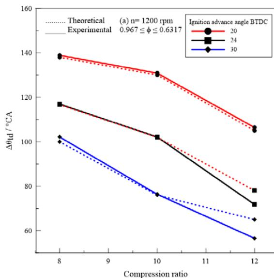
**Figure 3a: Effect of compression ratio on combustion total duration (1200 rpm).**
