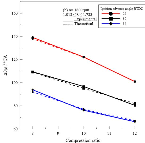
**Figure 3b: Effect of compression ratio on combustion total duration (1800 rpm).**
