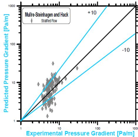
**Figure 18: Comparison between Experimental and Muller-Steinhagen and Heck Predictions (stratified flow)**
