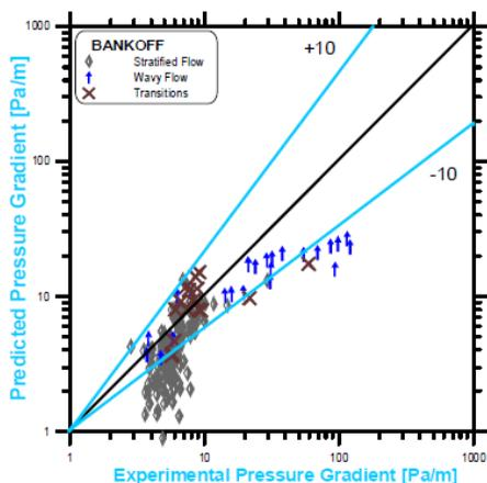
**Figure 8: Comparison between Experimental and Bankoff Predictions (Stratified, Wavy and Transition)**
