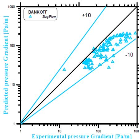
**Figure 20: Comparison between Experimental and Bankoff Predictions (slug flow)**
