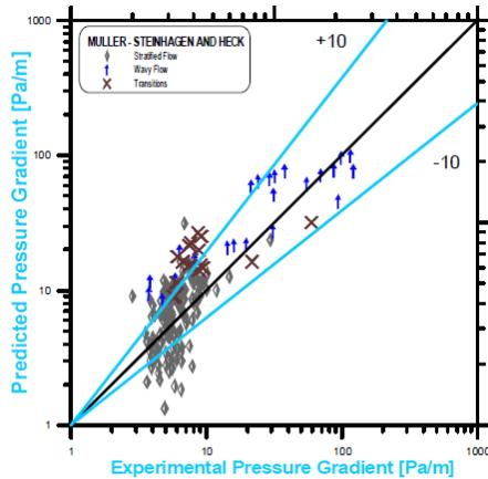
**Figure 12: Comparison between Experimental and Muller-Steinhagen and Heck Predictions (Stratified, Wavy and Transition)**
