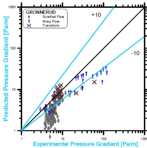
**Figure 10: Comparison between Experimental and Gronnerud Predictions (Stratified, Wavy and Transition)**
