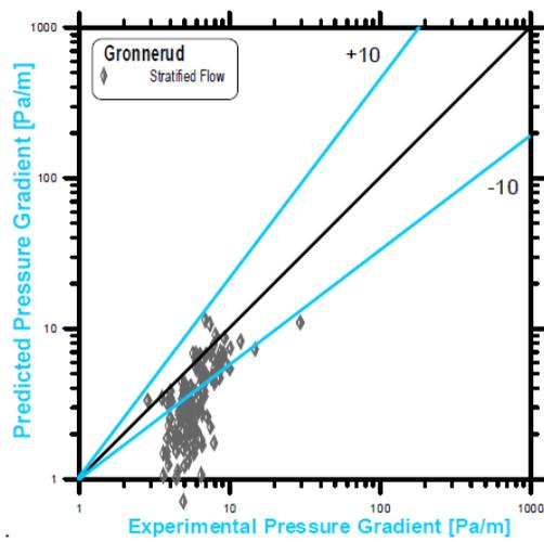
Figure 16: Comparison between Experimental and Gronnerud Predictions (stratified flow)
