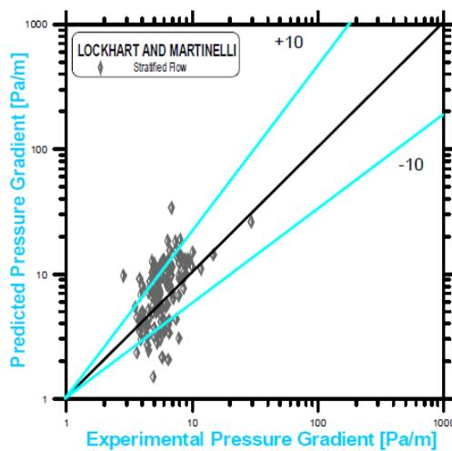
Figure 17: Comparison between Experimental and Lockhart and Martinelli Predictions (stratified flow)
