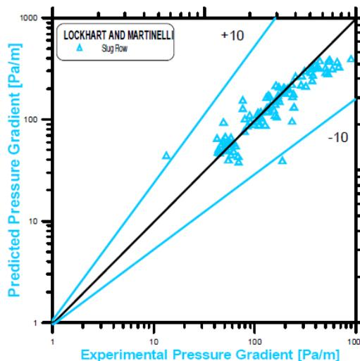
Figure 23: Comparison between Experimental and Lockhart and Martinelli Predictions (slug flow)
