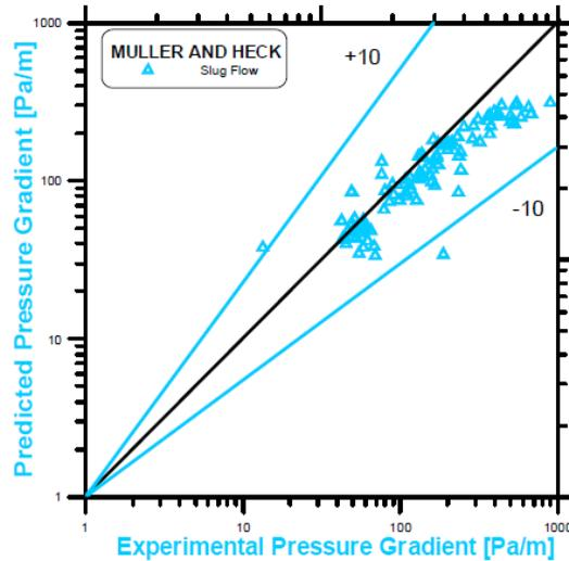
**Figure 24: Comparison between Experimental and Muller-Steinhagen and Heck Predictions (slug flow)**
