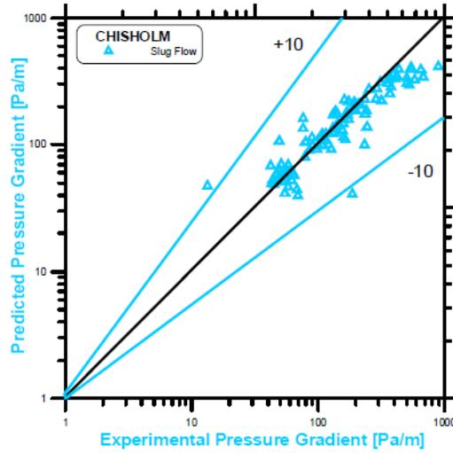
Figure 21: Comparison between Experimental and Chisholm Predictions (slug flow)
