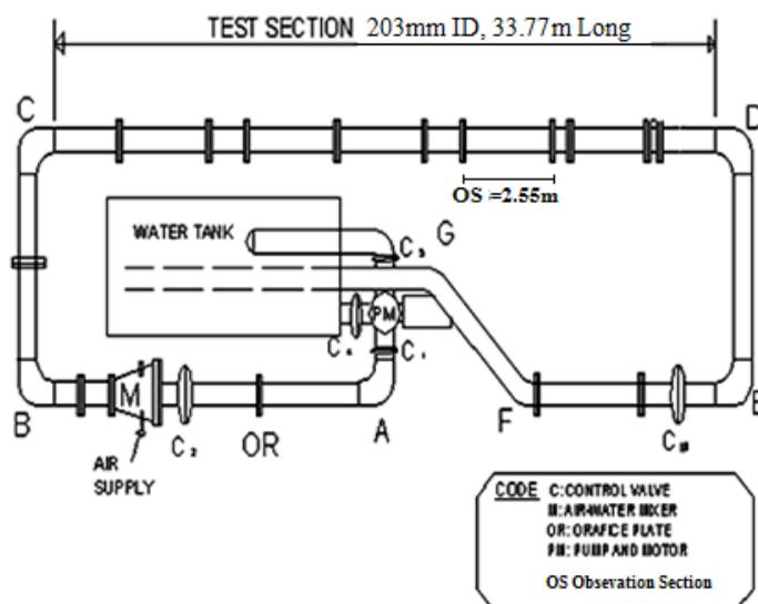
Figure 1: Layout of test rig [1].
