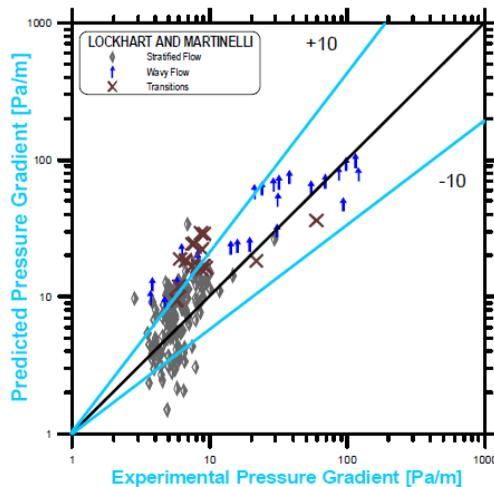
**Figure 11: Comparison between Experimental and Lockhart and Martinelli Predictions (Stratified, Wavy and Transition)**
