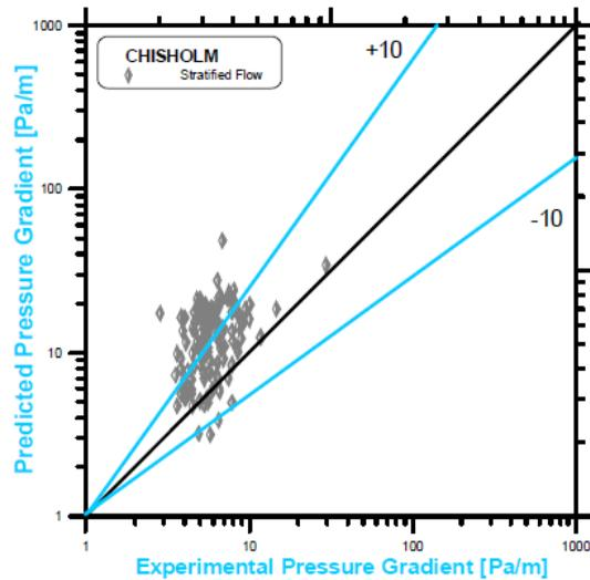
Figure 15: Comparison between Experimental and Chisholm Predictions (stratified flow)
