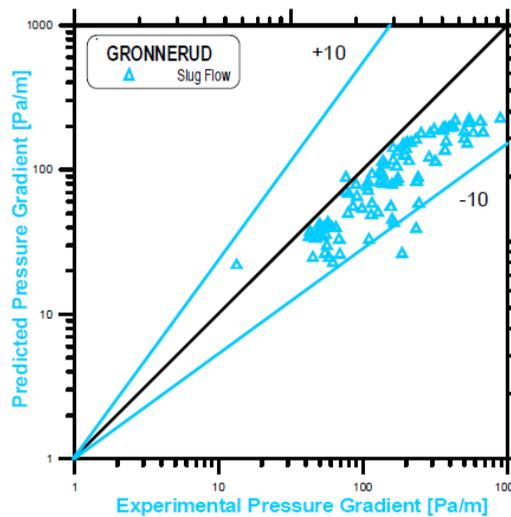
Figure 22: Comparison between Experimental and Gronnerud Predictions (slug flow)
