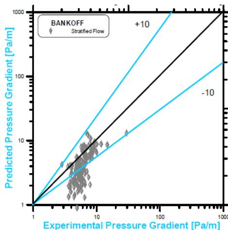
**Figure 14: Comparison between Experimental and Bankoff Predictions (stratified flow)**
