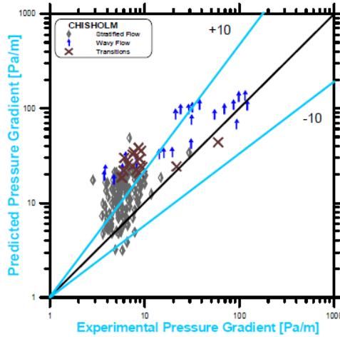
**Figure 9: Comparison between Experimental and Chisholm Predictions (Stratified, Wavy and Transition)**
