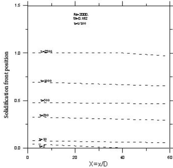
Figure 7: Location of solidification front in the axial direction
