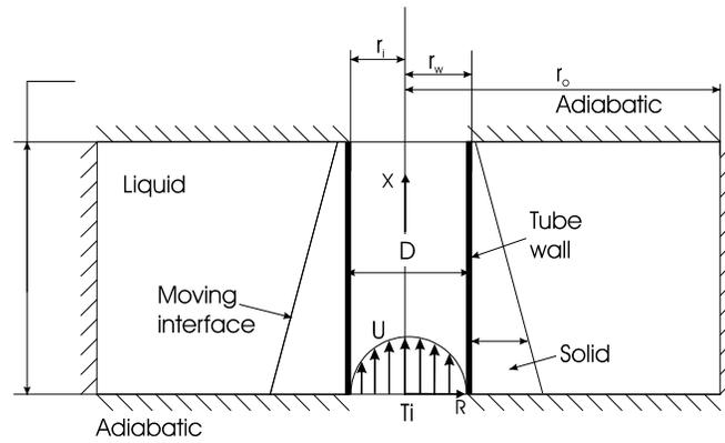
**Figure 2: Schematic diagram of the PCM thermal system**
