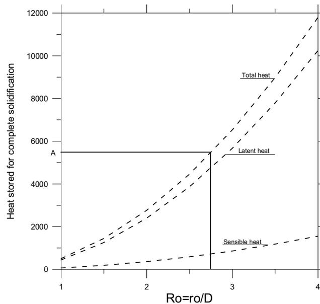
**Figure 11: Heat accumulated versus the outer radius of solidification.**
