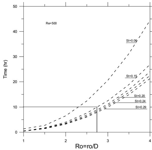
**Figure 10: Time cycle versus outer radius for different Stefan numbers**
