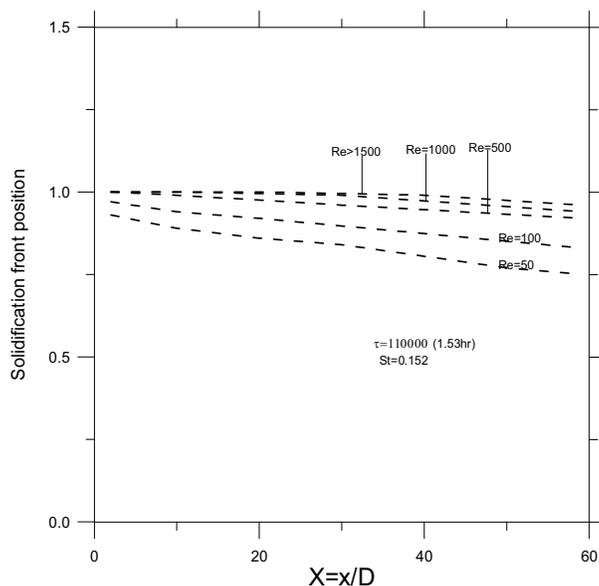
**Figure 8: Position of the solidification front for different Reynolds numbers.**
