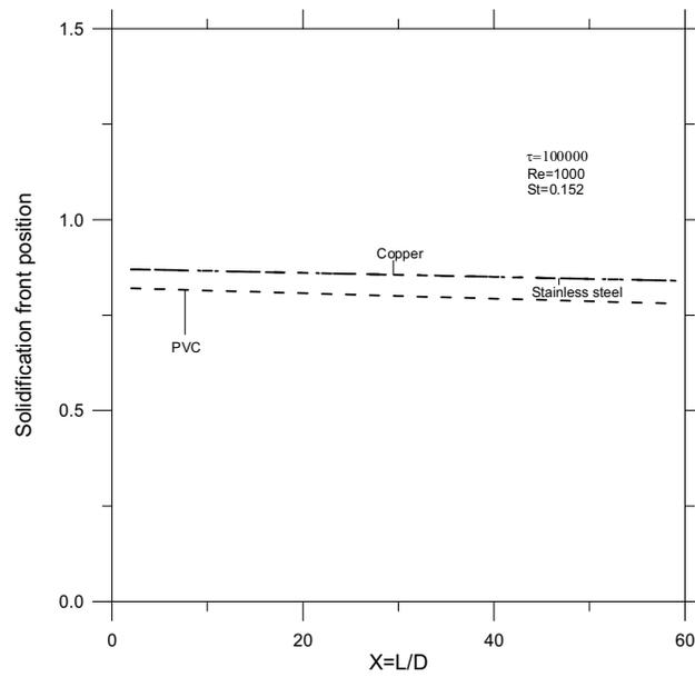
**Figure 9: Position of the solidification front for different tube wall material.**
