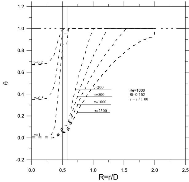
Figure 6: radial temperature distribution at the middle of the pipe.
