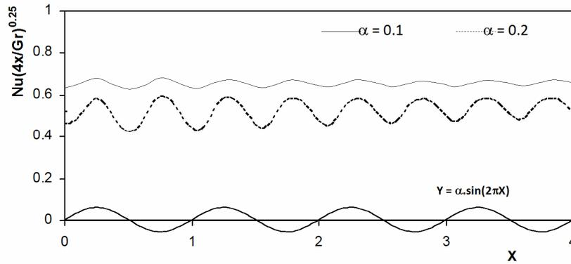
Figure 6: Local heat transfer rate for various amplitude wavelength ratios of wavy surfaces ( $\alpha = 0.1, 0.2$ , at  $Pr = 1.0$ ).
