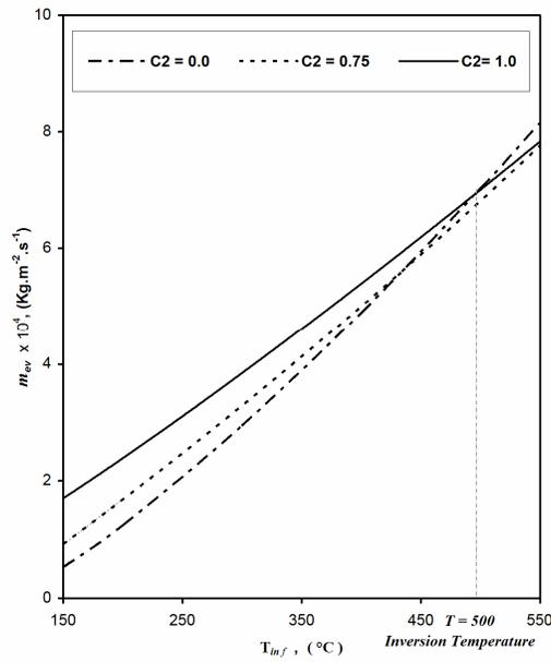
**Figure 7: Evaporation rate of water from vertical flat surface ( $\alpha = 0.0$ ) into various of free stream mass fraction.**
