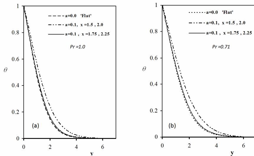
Figure 2: Temperature distribution ( $\theta$ ) for flat and wavy surface, (a)  $Pr=1.0$ , (b)  $Pr=0.71$ .
