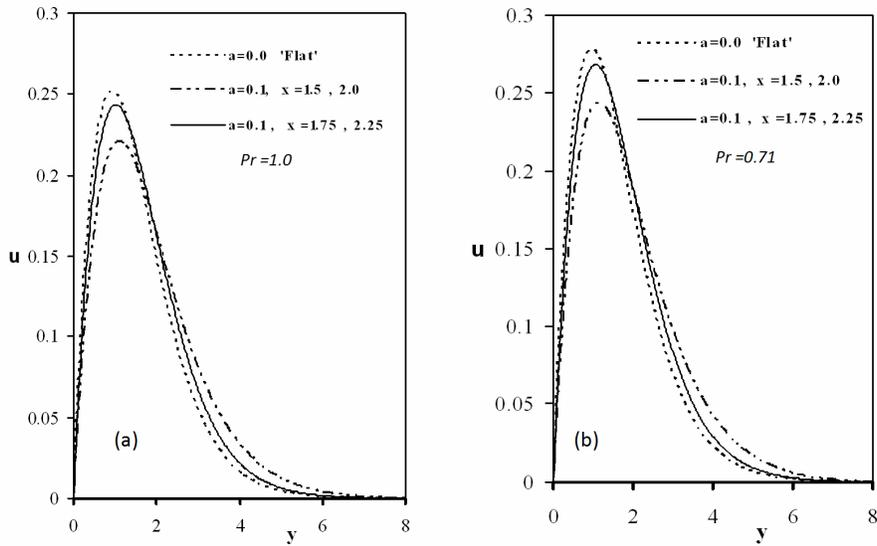
Figure 4: Axial velocity profiles ( $u$ ) for flat and wavy surface; (a)  $Pr=1.0$ , (b)  $Pr=0.71$ .
