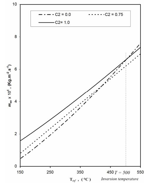
**Figure 8: Evaporation rate of Water from vertical wavy surface ( $\alpha = 0.2$ ) into various of ambient mass fraction.**
