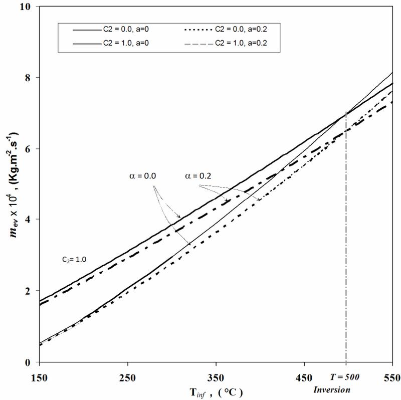
**Figure 9: Evaporation rate of Water from vertical flat and wavy surfaces ( $\alpha = 0.0, 0.2$ ) in pure air and super heated vapor.**
