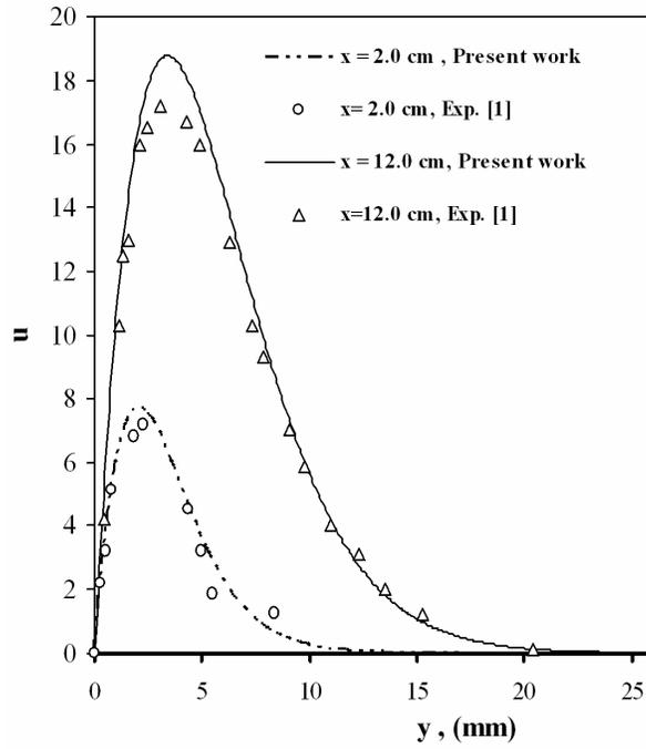
Figure 5: Dimensional Axial Velocity distribution ( $u$ ) for vertical flat surface ( $\alpha=0$ ), at  $x = 2.0$  cm and  $x = 12.0$  cm
