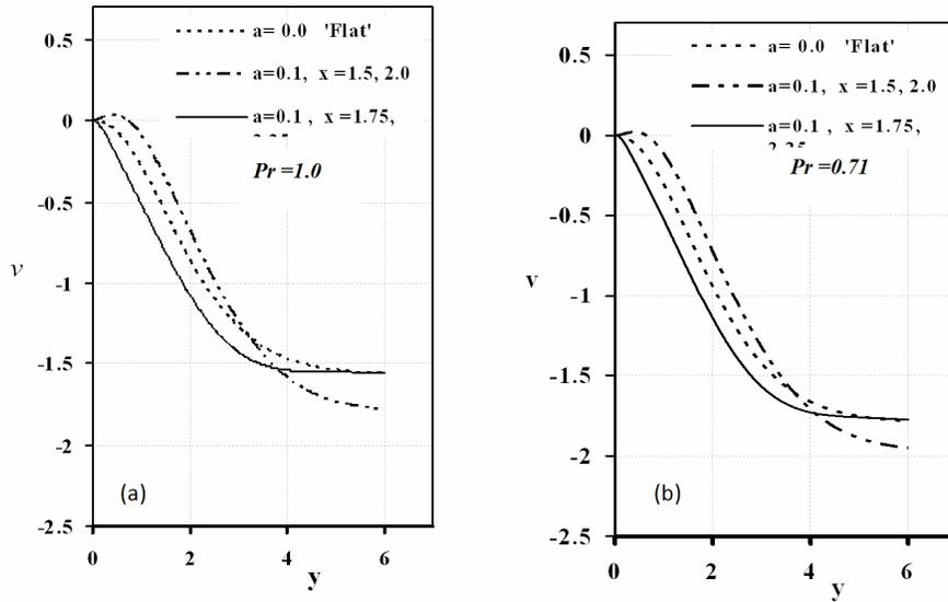
Figure 3: Normal velocity profiles ( $v$ ) for flat and wavy surface, (a)  $Pr=1.0$ , (b)  $Pr=0.71$ .
