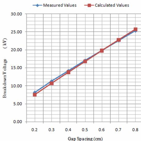
**Figure 5: Measured and calculated breakdown voltage.**
