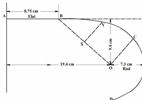
Figure 3: Half-contour of uniform field electrode used by Bruce [26]
