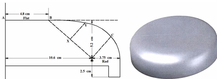
**Figure 4: Half-contour of uniform field electrode prototype designed (in cm), and AutoCAD isometric of the uniform field gap**
