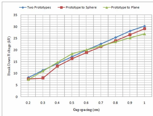
**Figure 8: B.D. Voltage between the Prototype sphere and different electrodes**
