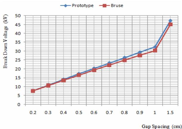
**Figure 6: Comparison between Bruce and the prototype Sphere**
