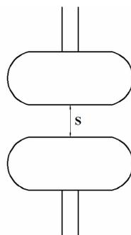
**Figure 1: Uniform field Electrodes**
