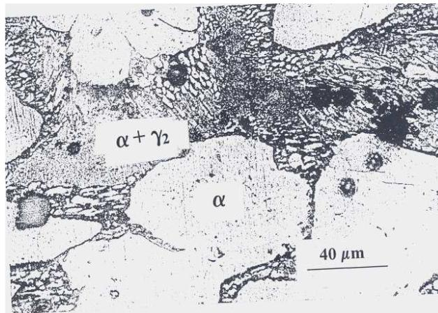
**Figure 2: Microstructure of as-annealed Cu-10.2 wt. % Al**
