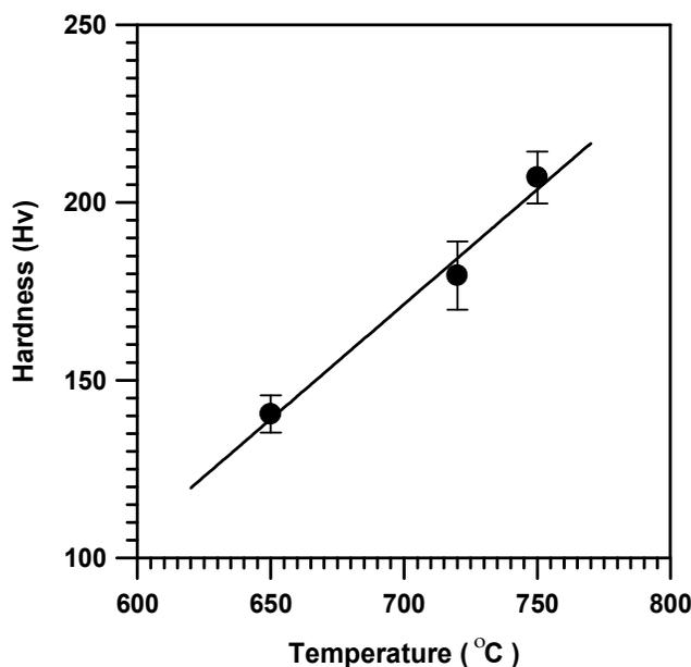
**Figure 4: Effect of equilibrating temperature on the overall hardness of dual-phase aluminum bronze**
