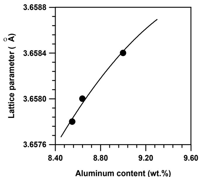
Figure 5: Effect of aluminum content on the lattice parameter of the  $\alpha$ -phase
