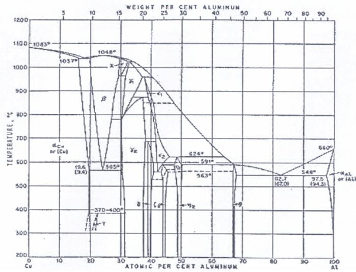
**Figure 1: The binary Cu-Al phase diagram**
