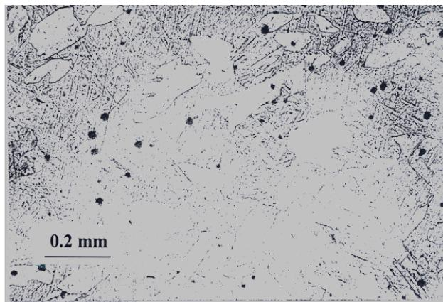
**Figure 3: A representative microstructure of the dual-phase structure obtained in Al-bronze after equilibration at 750°C followed by brine quenching**
