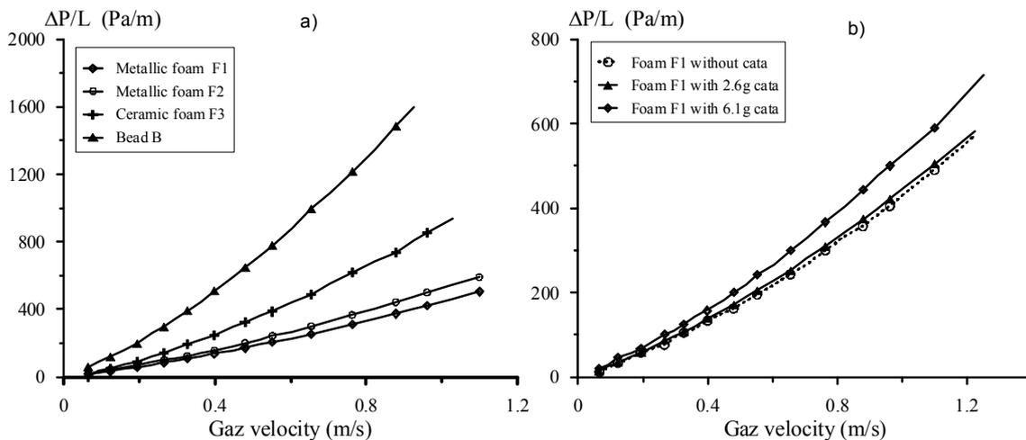
**Figure 4: Comparison of pressure drops foams and bead with and without catalyst. (a) Effect of catalyst loading. (b) Effect of structures**
