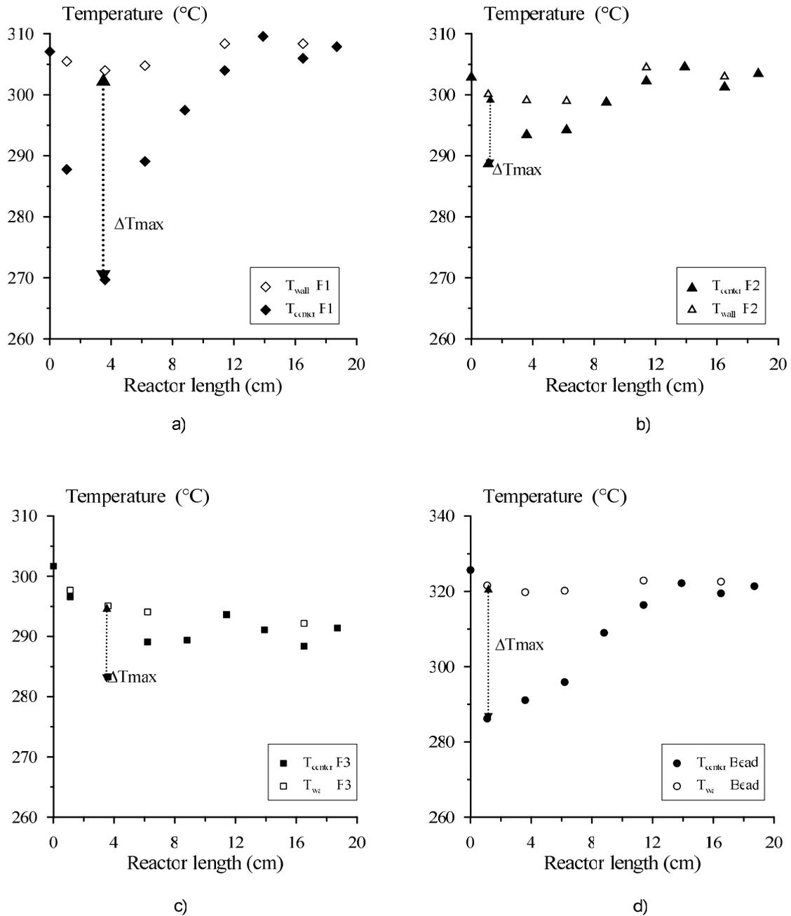
**Figure 7: Axial temperature profile for foams types and bead bed reactor at  $W/F_{MCH}$  of 15.3 kg<sub>cata</sub>.s.mol<sup>-1</sup> and at  $T_I=300^\circ\text{C}$ : a) Foam F1, b) Foam F2, c) Foam F3, d) Bead B.**
