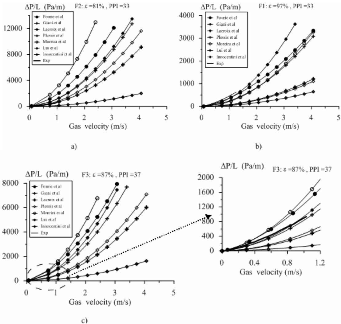
**Figure 5: Comparison of pressure drop results determined by different models with experimental data: a) F2:  $\varepsilon=87\%$  , ppi =33, b) F1:  $\varepsilon=97\%$  , ppi =33, c) F3:  $\varepsilon=87\%$ , ppi =37**
