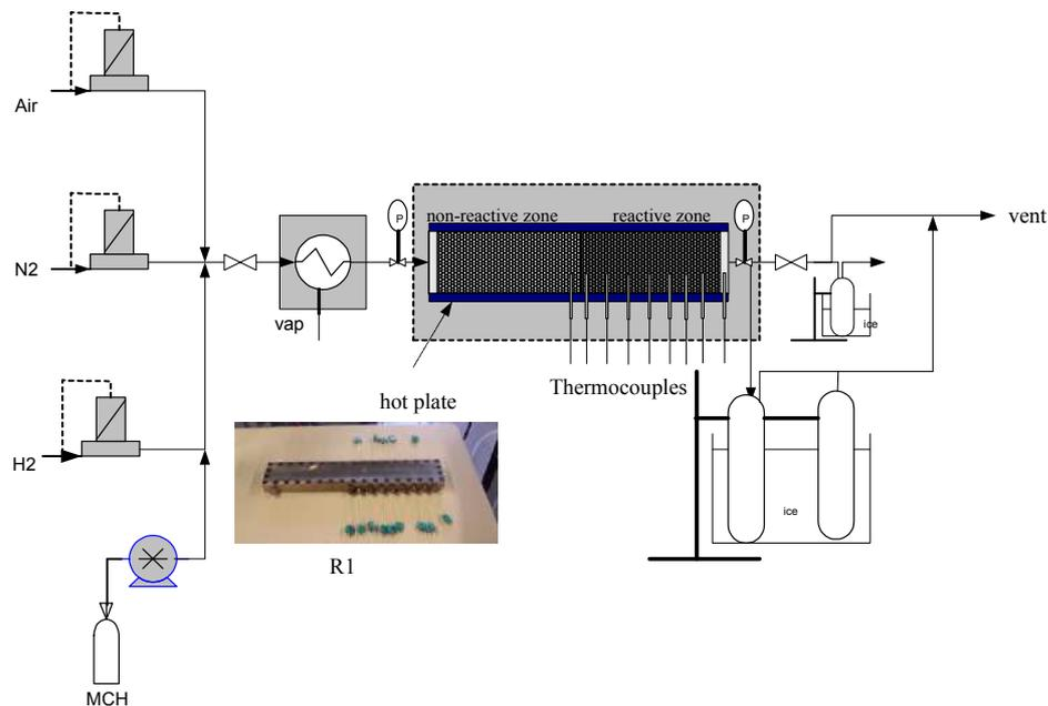
**Figure 3: Experimental setup used for catalyst testing**
