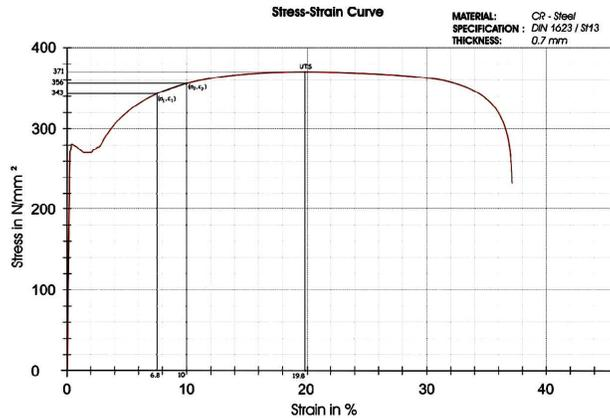
Figure 8: The Stress Strain curve for "Mat1".
