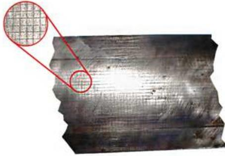
**Figure 3: The drawing grid on the drawn part**
