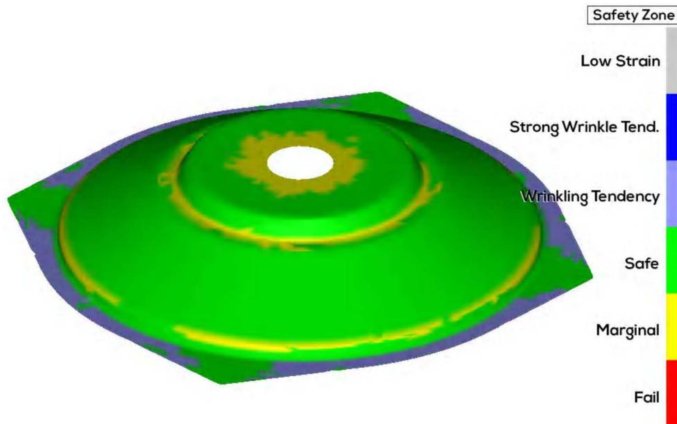
**Figure 11: Safety zone contour for "Mat-2" after forming.**
