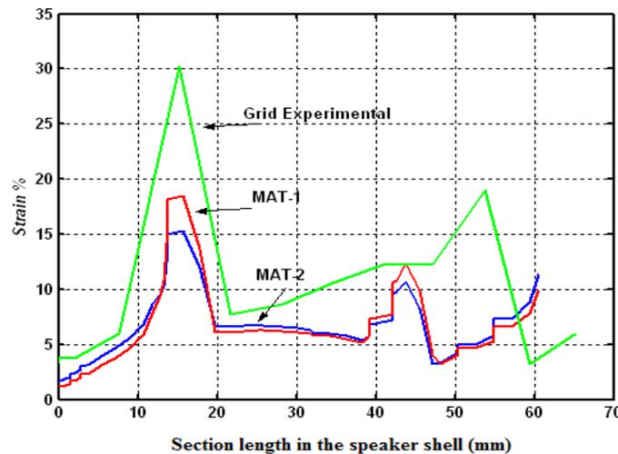
Figure 9: Long diameter strain distribution for "Mat-1", "Mat-2" and the measured ones.
