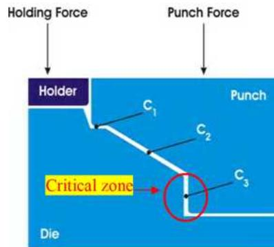
**Figure 6: The clearance between punch and die**
