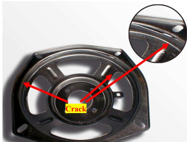
**Figure 12: The cracks resulted at critical zones.**
