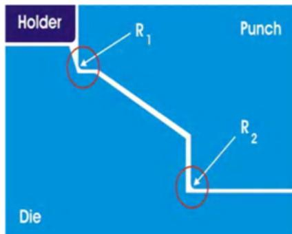
**Figure 7: The radius of drawing punch at two critical points**
