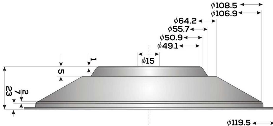
**Figure 1: The dimensions of the speaker shell in (mm)**
