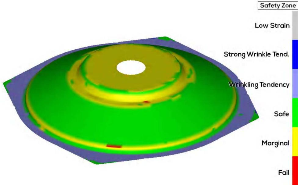
**Figure 10: A safety zone contour for "Mat-1" after forming.**
