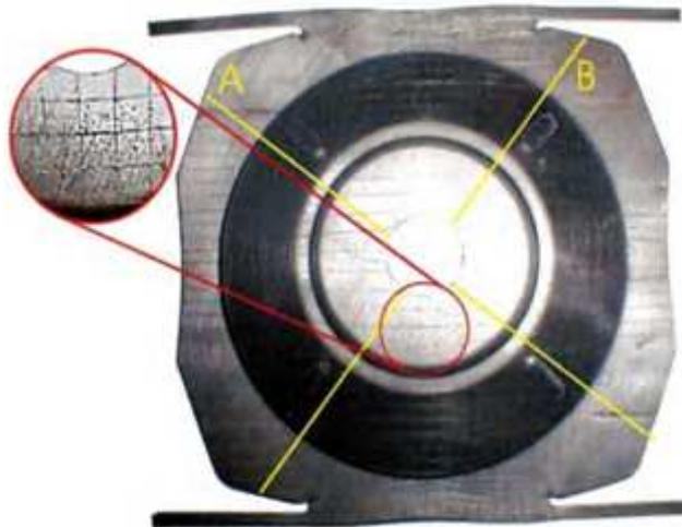
**Figure 2: The drawing grid on the blank surface**
