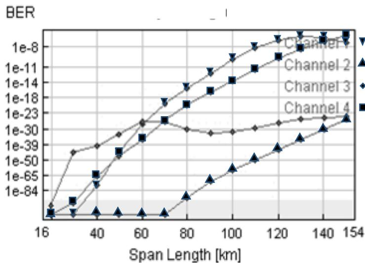
Figure 11: As the span length increases, XPM becomes more severe.
