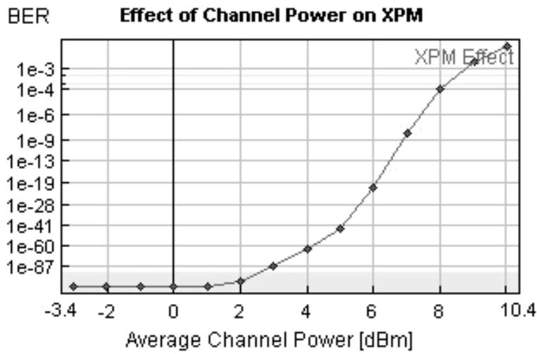
**Figure 9: Effect of channel power on XPM**
