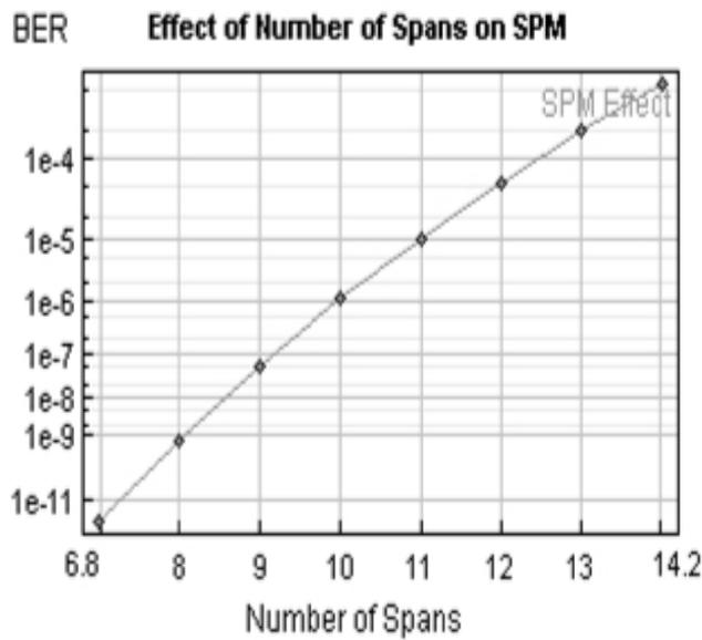
**Figure 7: Effect of number of amplifier spans on SPM**
