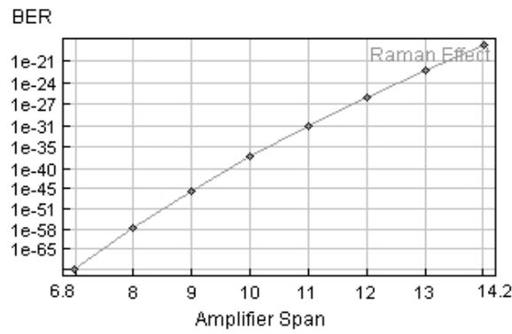
**Figure 4: Effect of number of amplifier spans on SRS**
