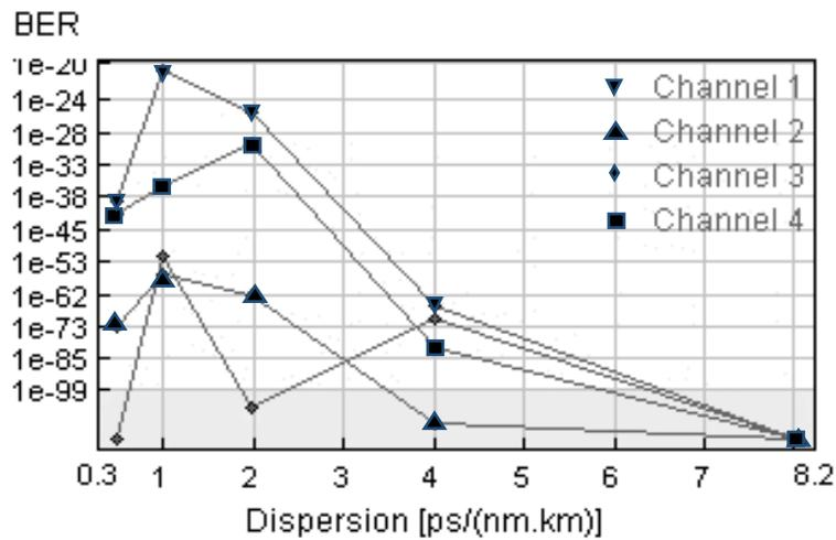
**Figure 10: Effect of dispersion on XPM**
