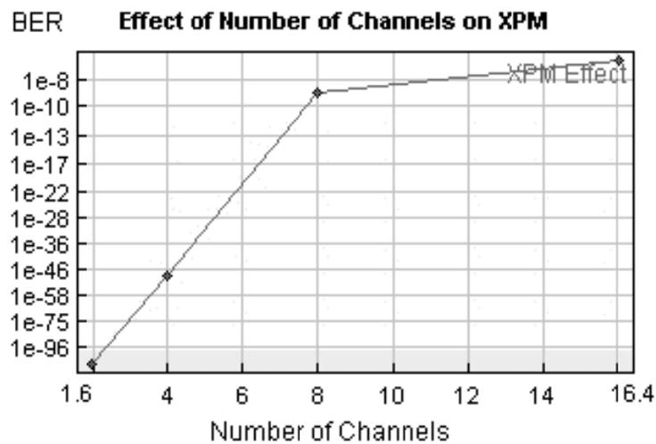
Figure 12: Effect of number of channels on XPM
