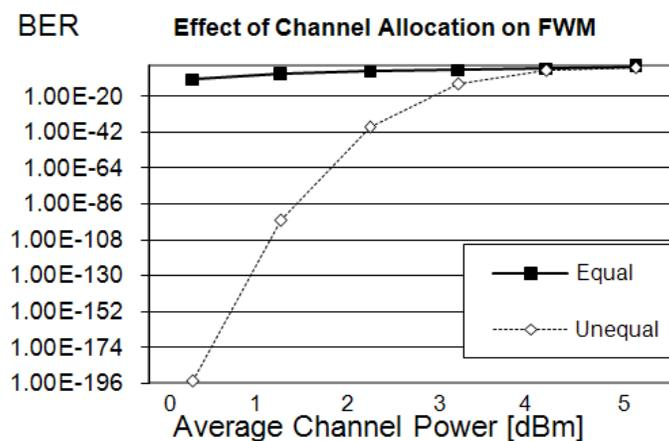
**Figure 16: Effect of channel allocation on FWM**
