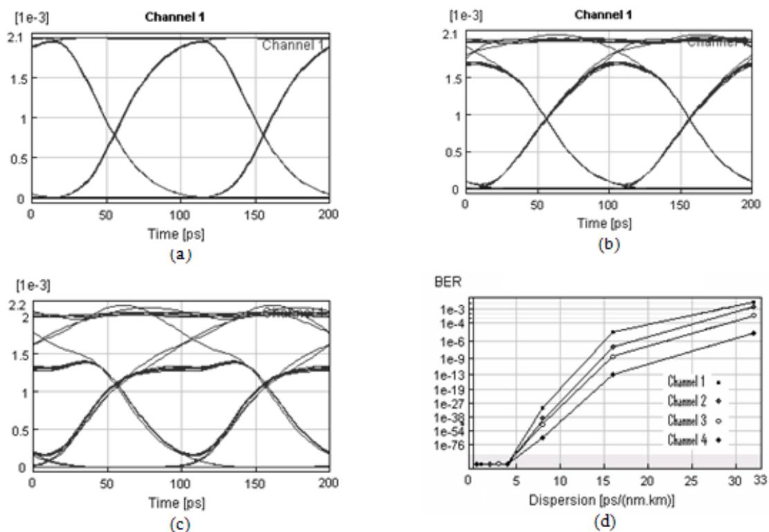
Figure 6: Effect of dispersion on SPM
