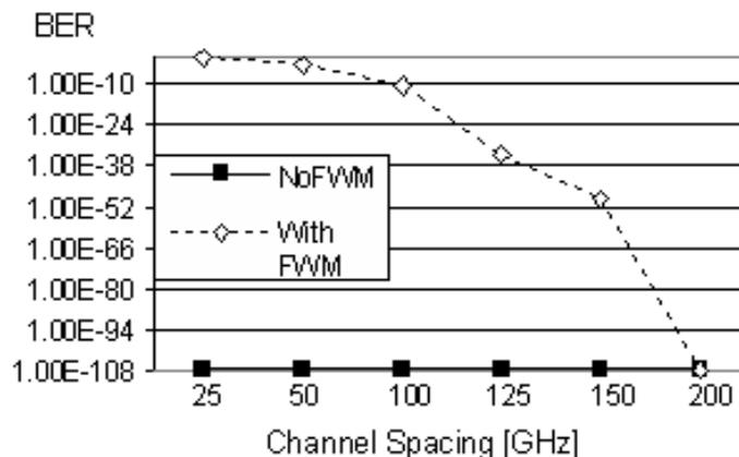
**Figure 14: Effect of channel spacing on FWM**
