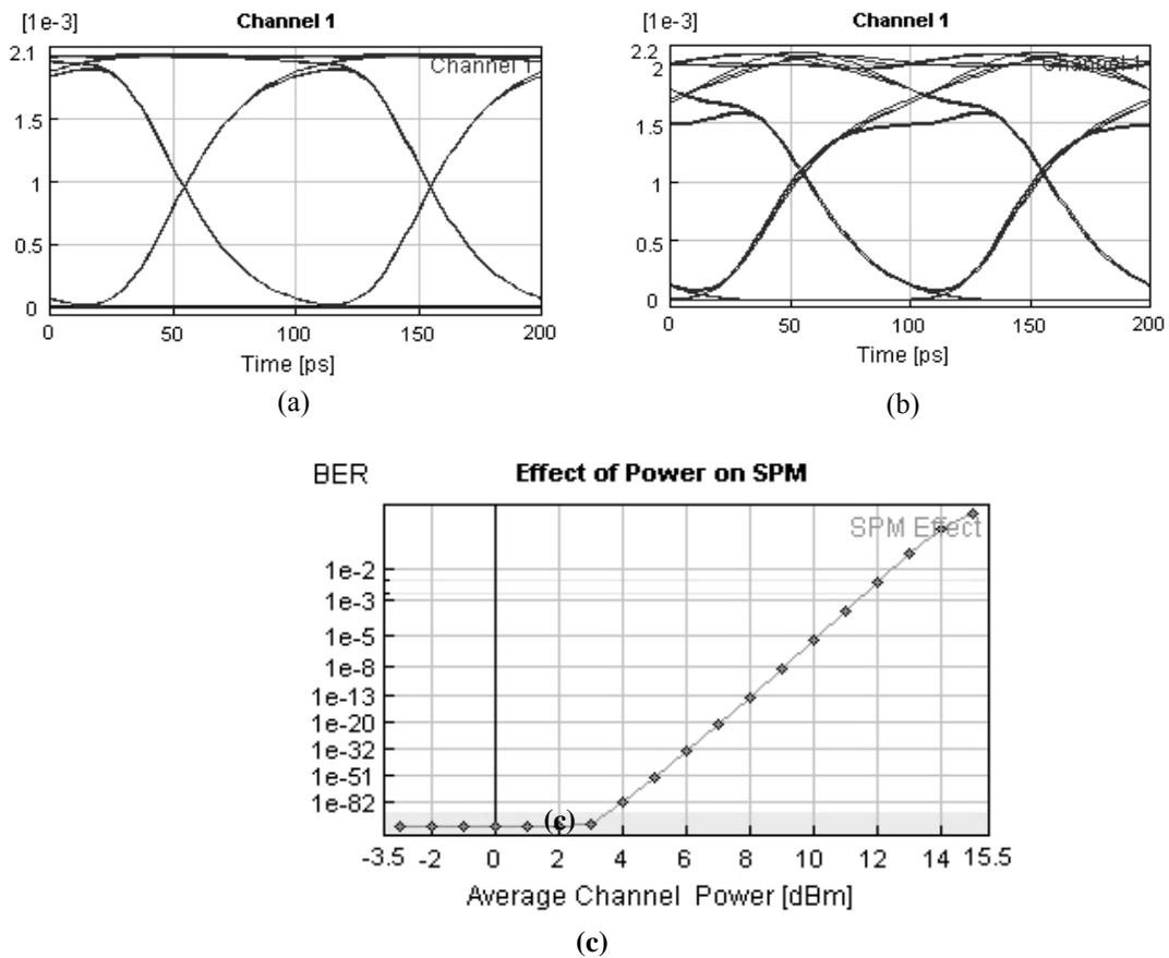
**Figure 5: Effect of Power on SPM**
