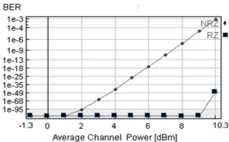
**Figure 8: Effect of modulation type on SPM**
