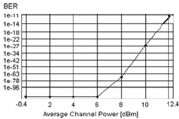
**Figure 2: the effect of power on SRS**
