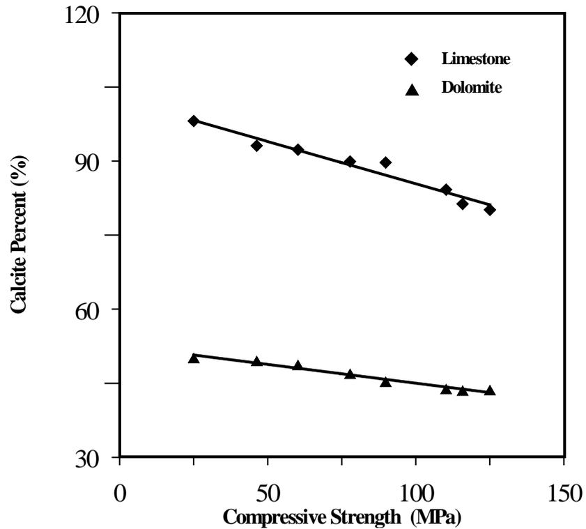
**Figure 2: Compressive strength and calcite weight percent relationship**
