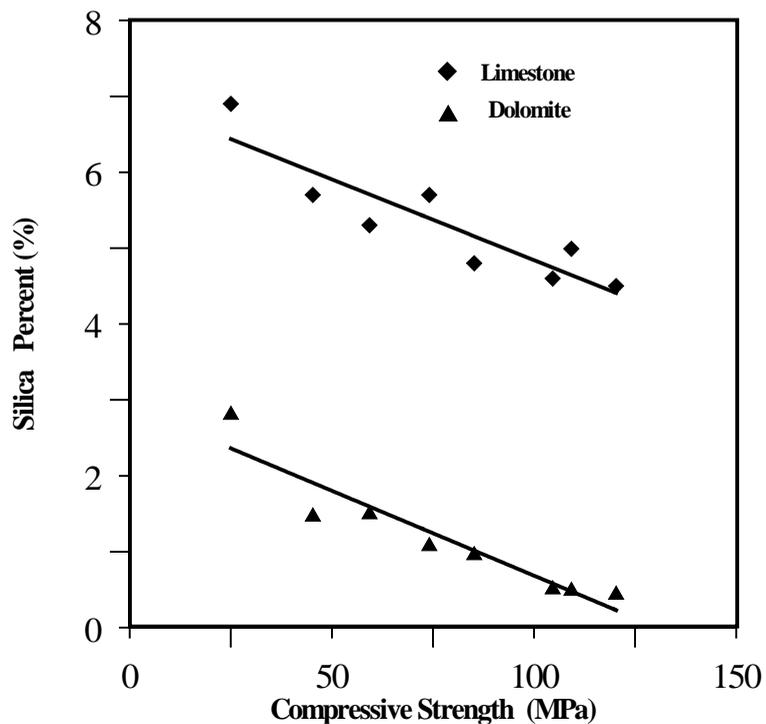
**Figure 3: Compressive strength and silica weight percent relationship**
