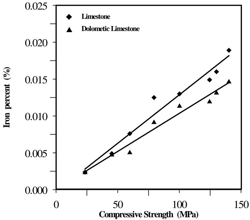
**Figure 4a: Compressive strength and iron weight percent relationship**
