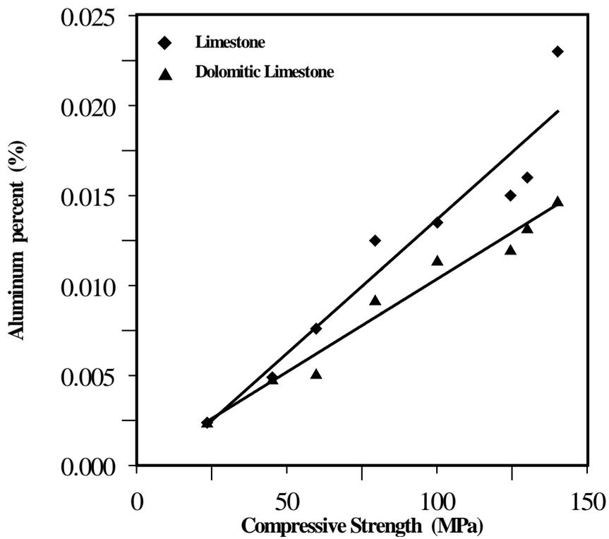
**Figure 4b: Compressive strength and aluminum weight percent relationship**
