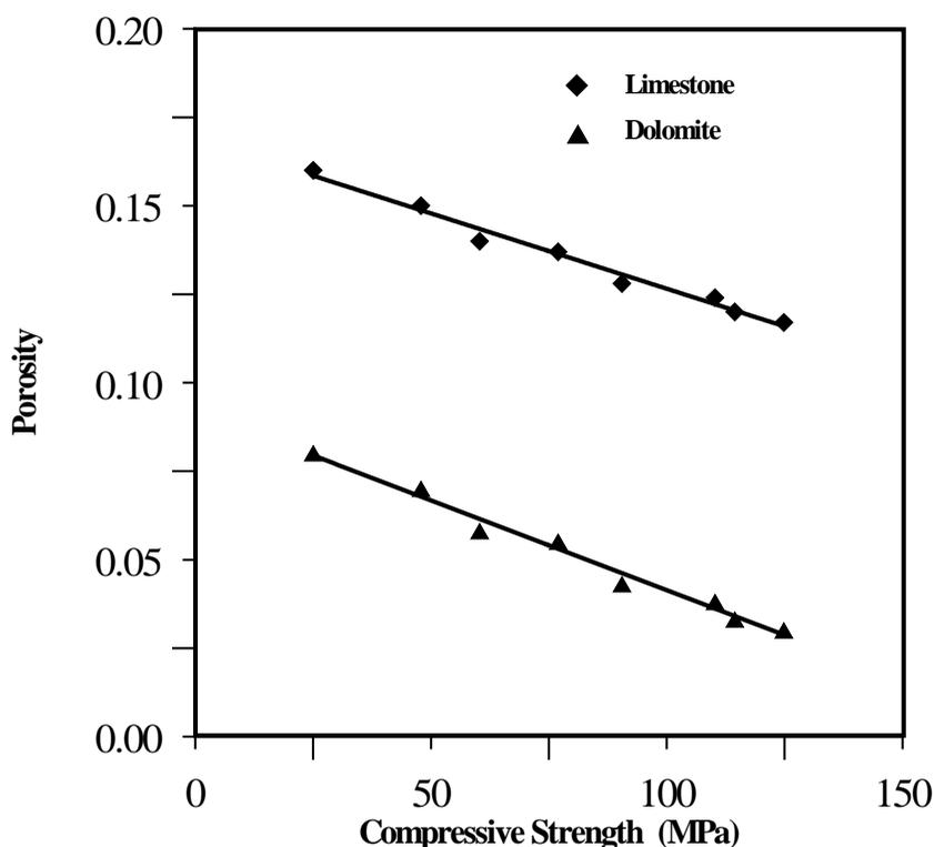
**Figure 5: Compressive strength and porosity relationship**
