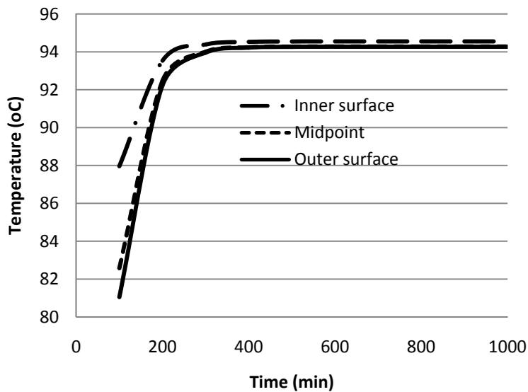
**Figure 3: Variation of temperature with time for cast iron in the middle of the storage unit**
