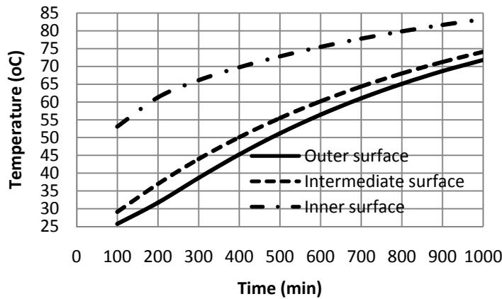
**Figure 4: Variation of temperature with time for brick in the middle of the storage unit**
