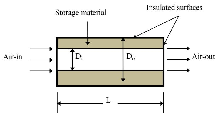
**Figure 1: Thermal energy storage unit**
