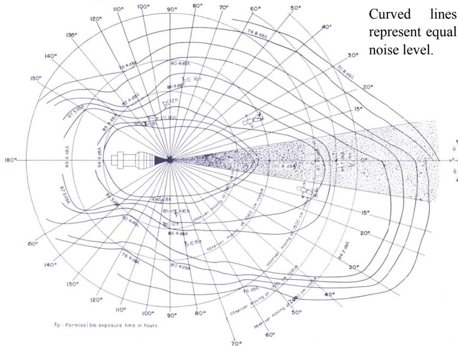
**Figure 5: Noise field from a jet engine aircraft at idling engine speed (40% r.p.m).**
