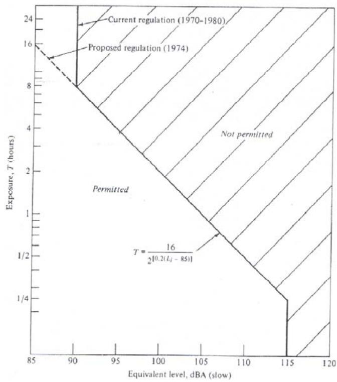
**Figure 4: Allowed exposure for continuous level, (OSHA), [2].**
