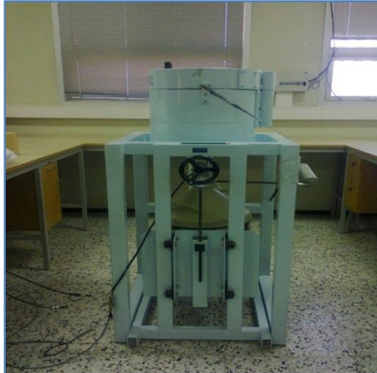
Figure 2: A photograph of the HPGe detector with accompanying lead castle used by the NRL.
