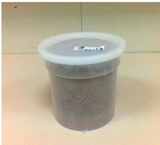
**Figure 1: A picture of the Marenelli beaker used in this study.**
