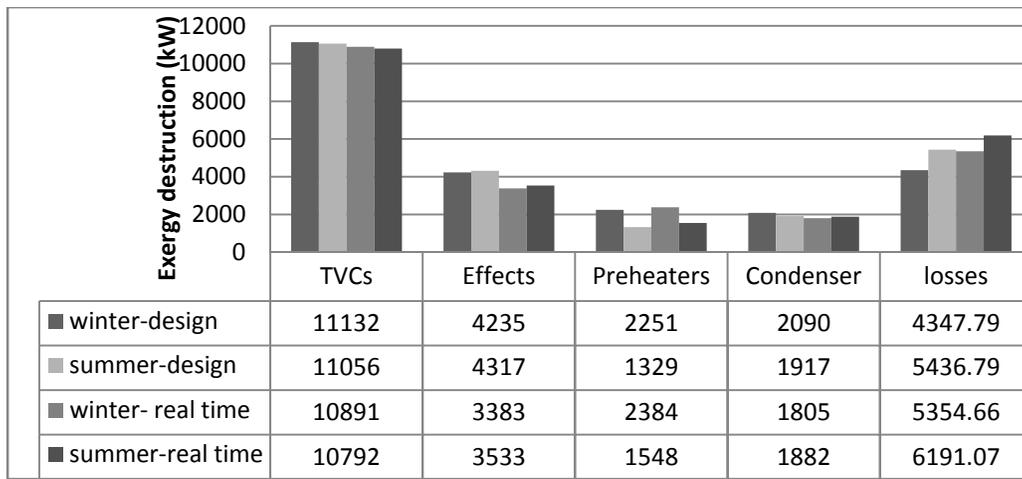
**Figure 5: Rate of Exergy destruction for different operating conditions**
