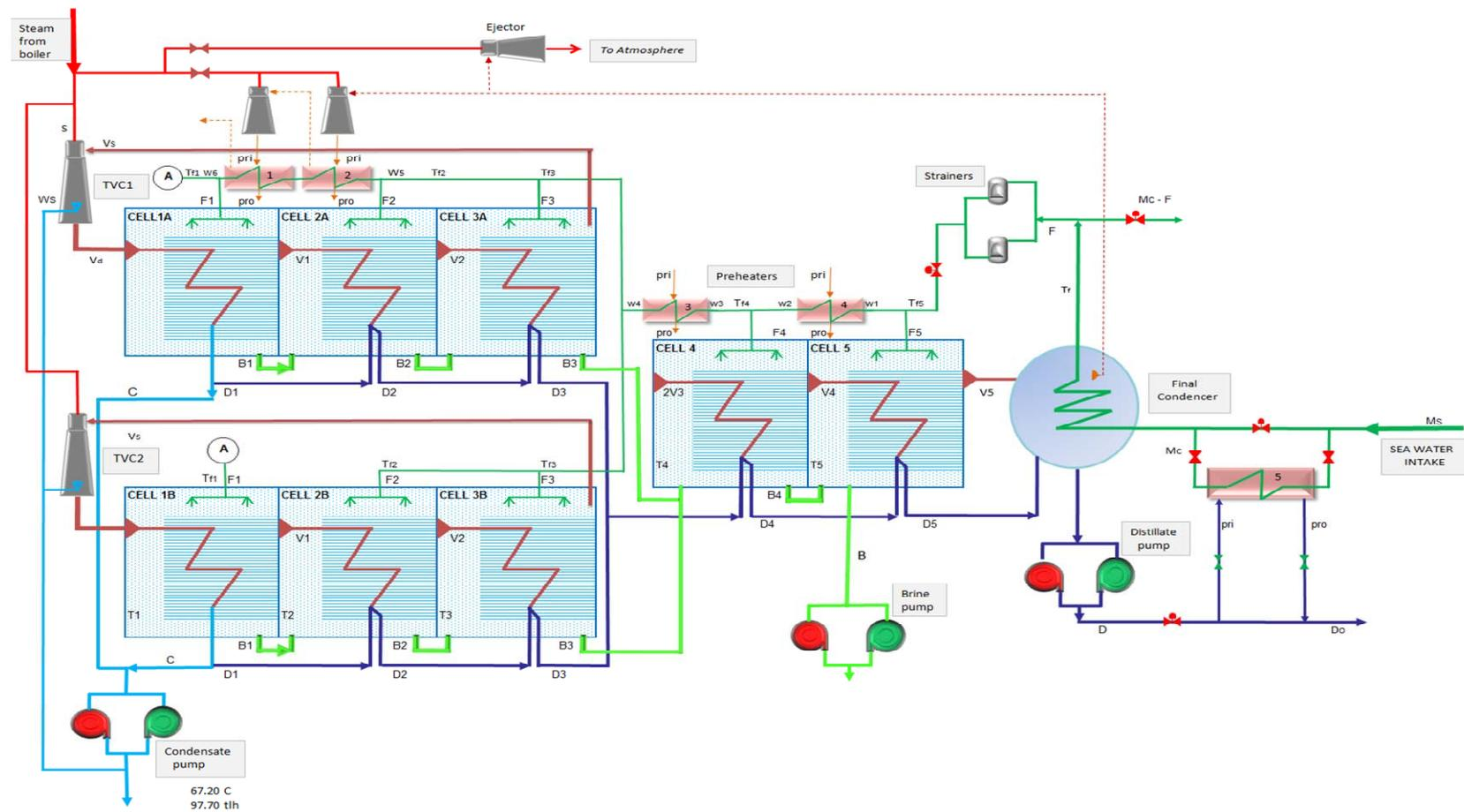
Figure 1: Schematic diagram for unit one of Zawia desalination plant
