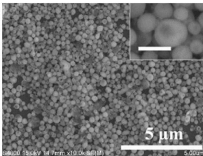
**Figure 4:** Shows the SEM image of pure iron nanoparticles, sample 6 (4 hrs., 20 ml)
