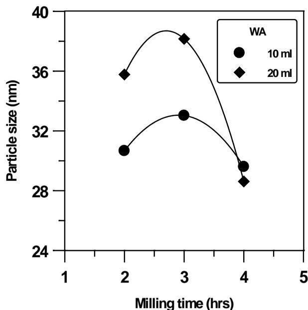
**Figure 5: The effect of milling time and WA on the particle size of milled powder**
