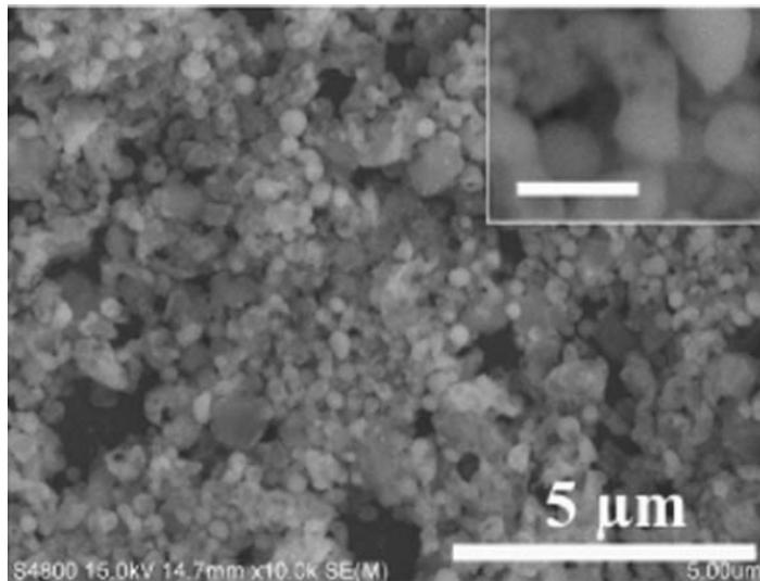
**Figure 3:** Shows the SEM image of pure iron nanoparticles, sample 2 (2 hrs, 20 ml)
